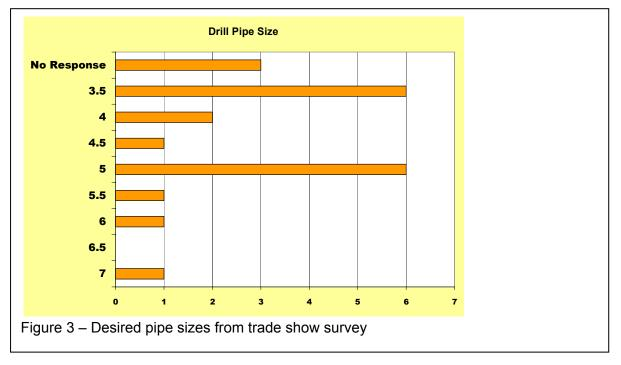
Although some trends are apparent, the small sample size does not give sufficient confidence that we have identified the optimum pipe size. As a generality, almost all interviewees were strongly in favor of the largest possible inside diameter, from both hydraulics and fishing tool requirements.
