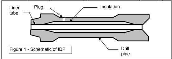
considered to be the same as that of the parent drill pipe; that is, the liner and insulation neither add to nor detract from the strength of the drill pipe. Mechanical testing was successfully completed at Stress Engineering Services in Houston in late 2007.
