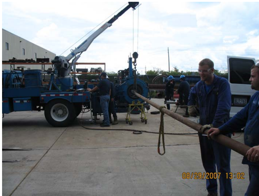
Pipe being made ready for torsion test. Truck mounted tongs applied torque to one end of pipe. Other end held to prevent rotation.
