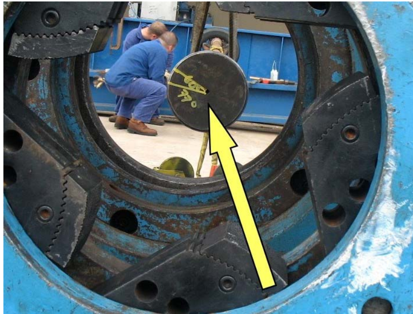
End of pipe before being gripped by tongs in torsion test. 77 degree mark, when vertical, indicates degrees rotation for torque of 33,413 ft-lbs, yield torque of pipe.
