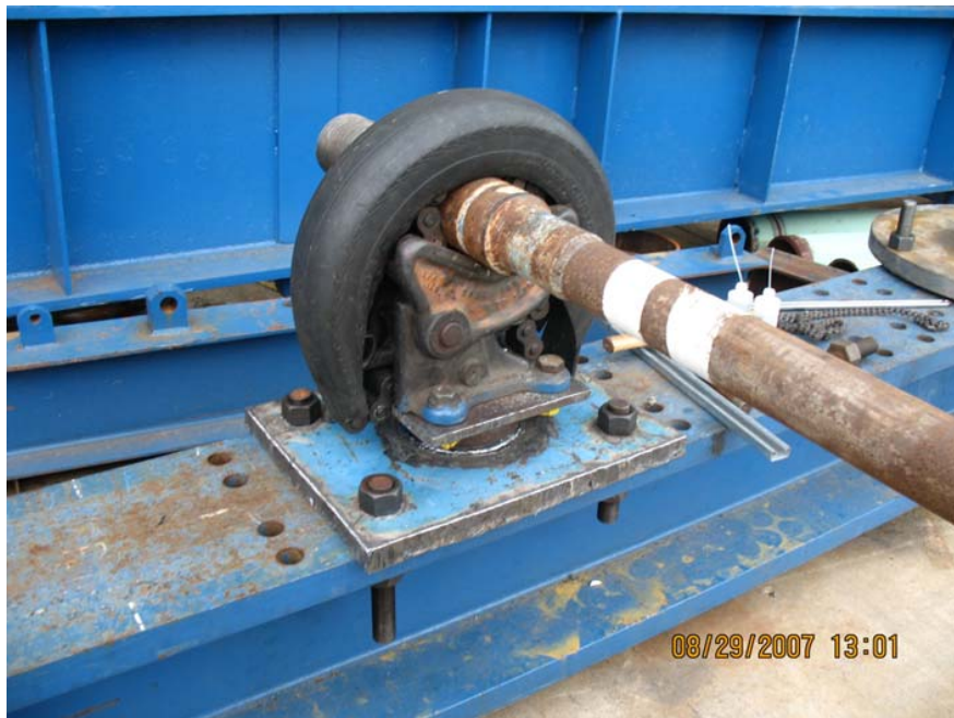
End of pipe in chain vise to prevent rotation during torsion test.
