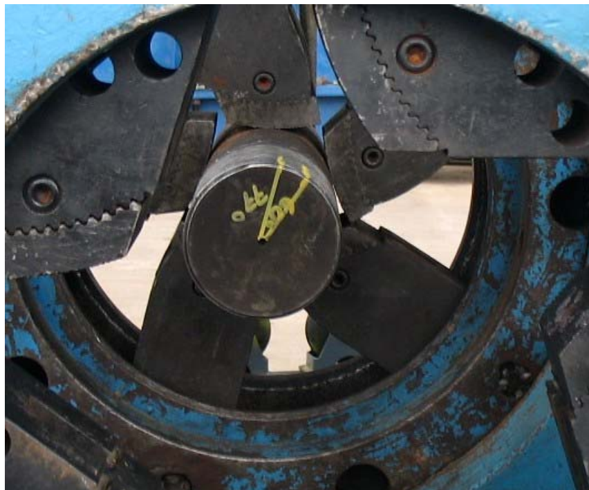
Final position of pipe during torsion test. Pipe had an angle of twist greater than 77 degrees which means it went beyond its torsional yield strength of 33,413 ft-lbs. No leakage at 200 psi occurred from the tool joint bore to the insulated annulus.
