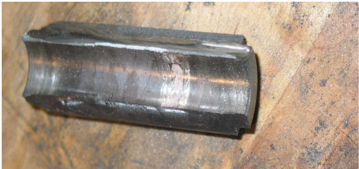
Figure 20: Section of planet gear showing wear
