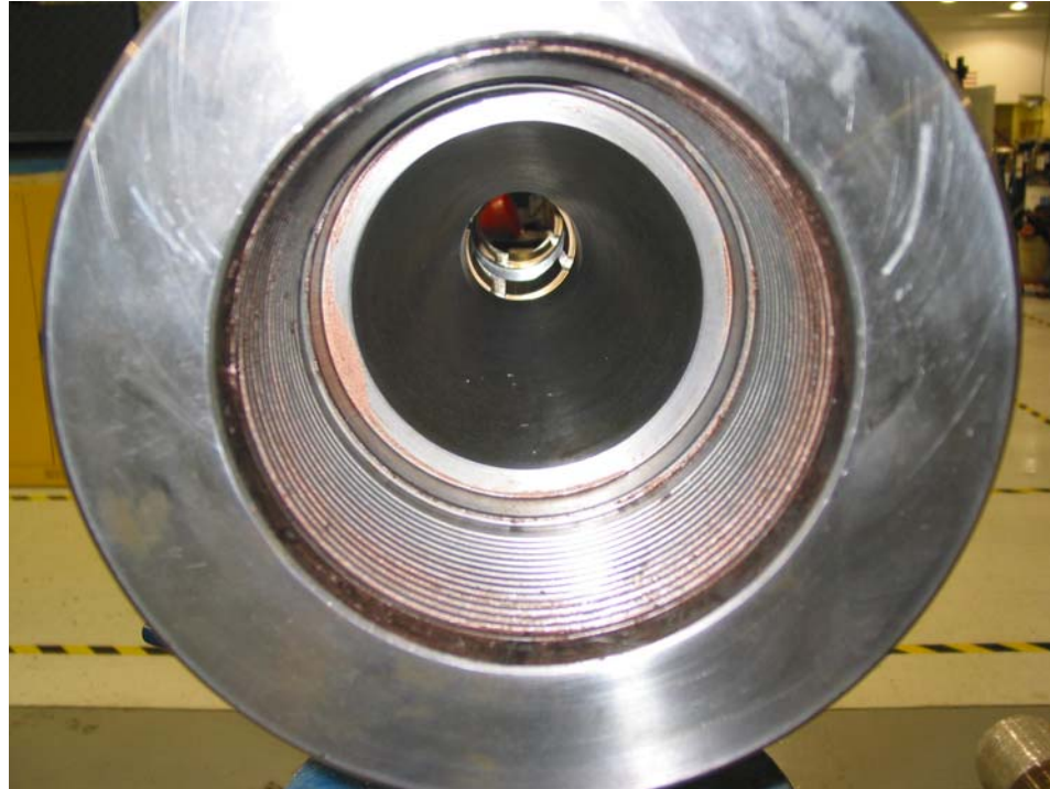
Figure 14: 'Vortex of Doom' to match angular velocities of mud and rotor
