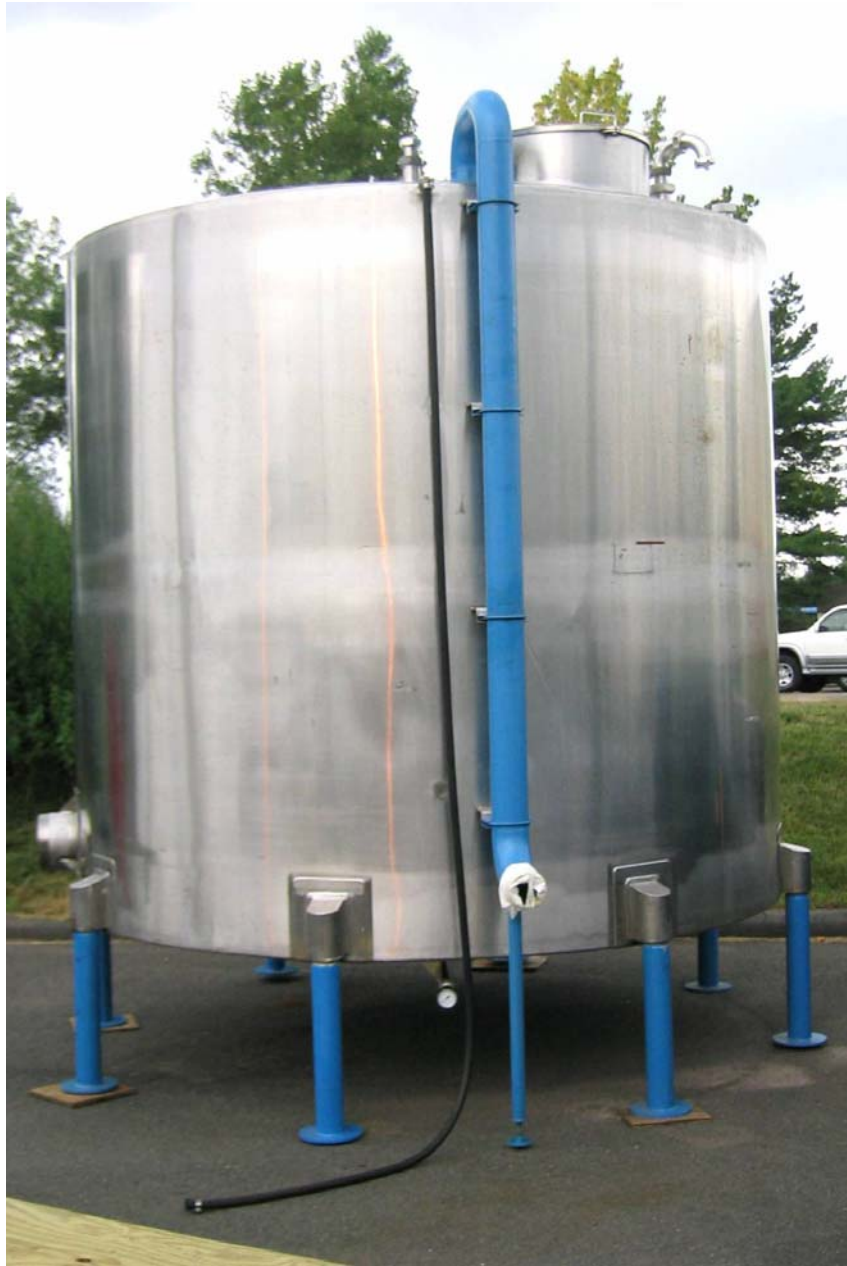
Figure 9: Storage tank (recycled from soda bottler)
