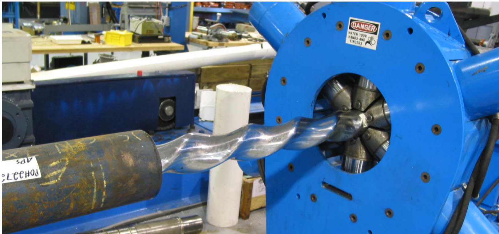
Figure 16: Installing the rotor in the power section
