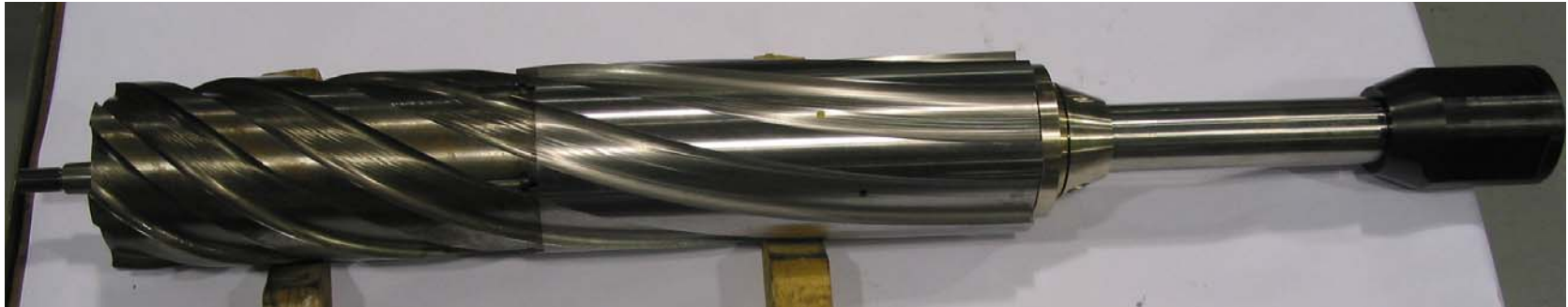
Figure 13: Variable pitch helical fin element
