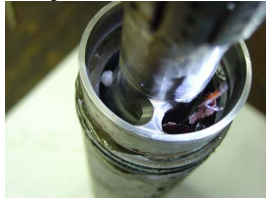
Figure 24: Debris (pipe scale) lodged within the BCPM. Disassembly after the BETA field trial.
