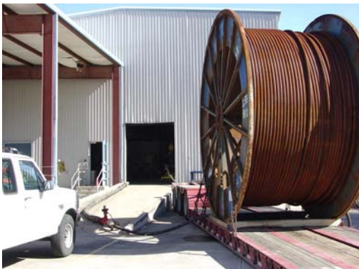
Figure 27: 7,000 foot coil inserted in flow loop. View towards test area.
