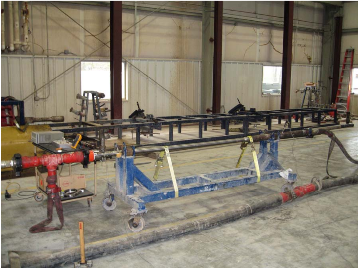
Figure 22: 2-3/8" BCPM operating in the Houston Flow Loop
