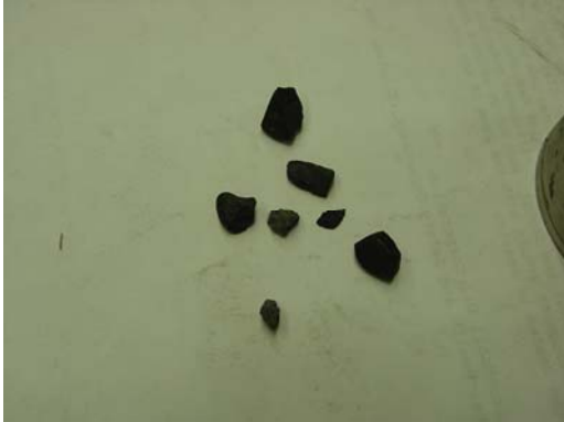
Figure 23: Debris extracted from inside the first BCPM during inspection in Houston, after the field trial at BETA
