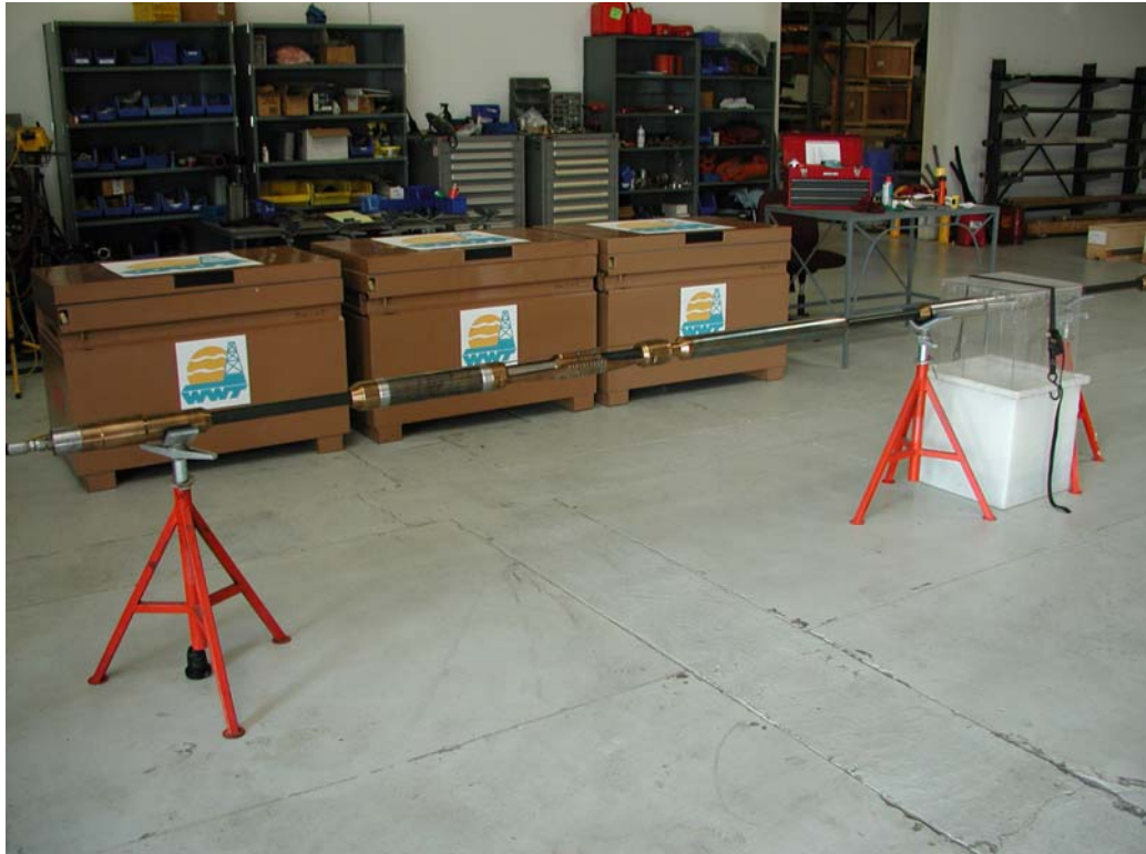
Photo 1: Approximately half of Microhole Drilling Tractor showing the Tool Joint (far left), Shaft Assembly with Gripper (center) and Control Assembly (far right)
