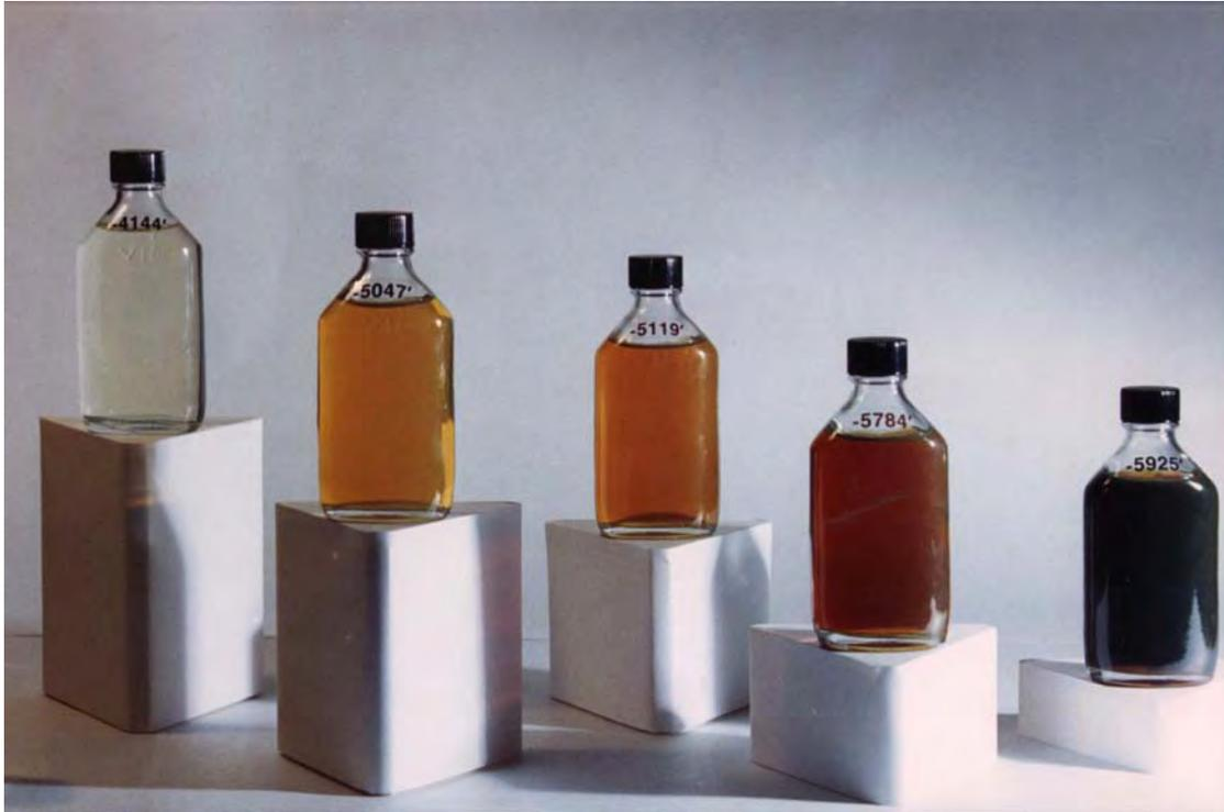
*Figure 3-22. Color changes in retrograde condensate from Anschutz Ranch East field, Summit County, Utah. Sample bottles are labeled with subsea structural elevation.*
