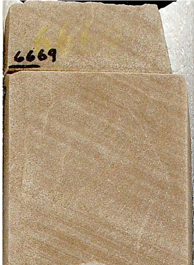
*Figure 5-6. Typical upper unit of the Navajo Sandstone, from the Kings Meadow Ranches No. 17-3 well (slabbed core from 6669 feet), Covenant field, showing cross-bedding in fine-grained sandstone deposited in a dune environment.*
