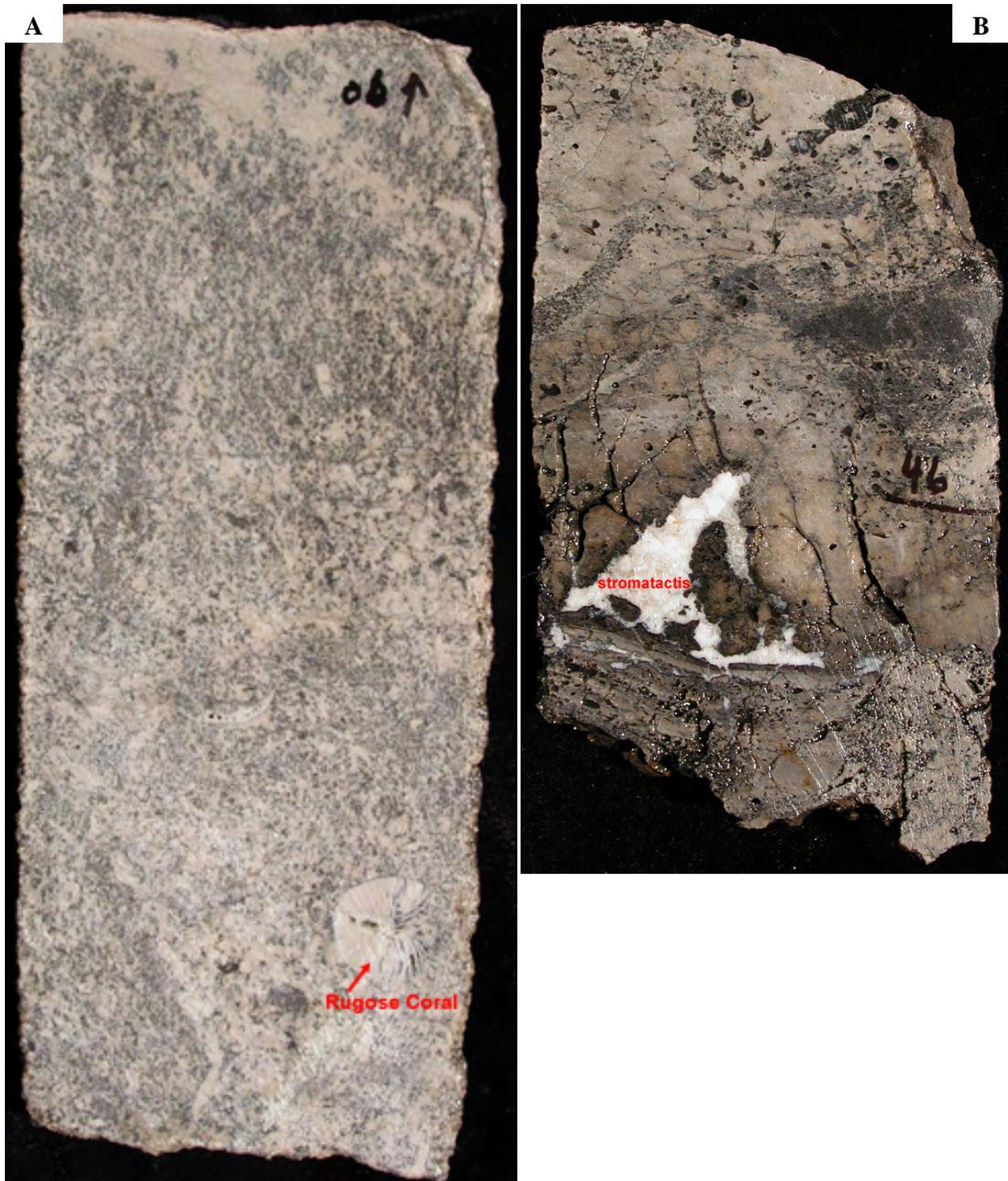
*Figure 9-6. Typical Leadville Limestone depositional fabrics from Lisbon field, San Juan County, Utah. A - Crinoidal/skeletal grainstone/packstones representing high-energy, open-marine shoal facies; slabbed core from 8506.5 feet, Lisbon No. B-816 well. B - Peloidal/skeletal packstone/wackestones representing moderate- to low-energy, open-marine, Waulsortian-type buildup facies; slabbed core from 8646 feet, Lisbon No. B-816 well.*
