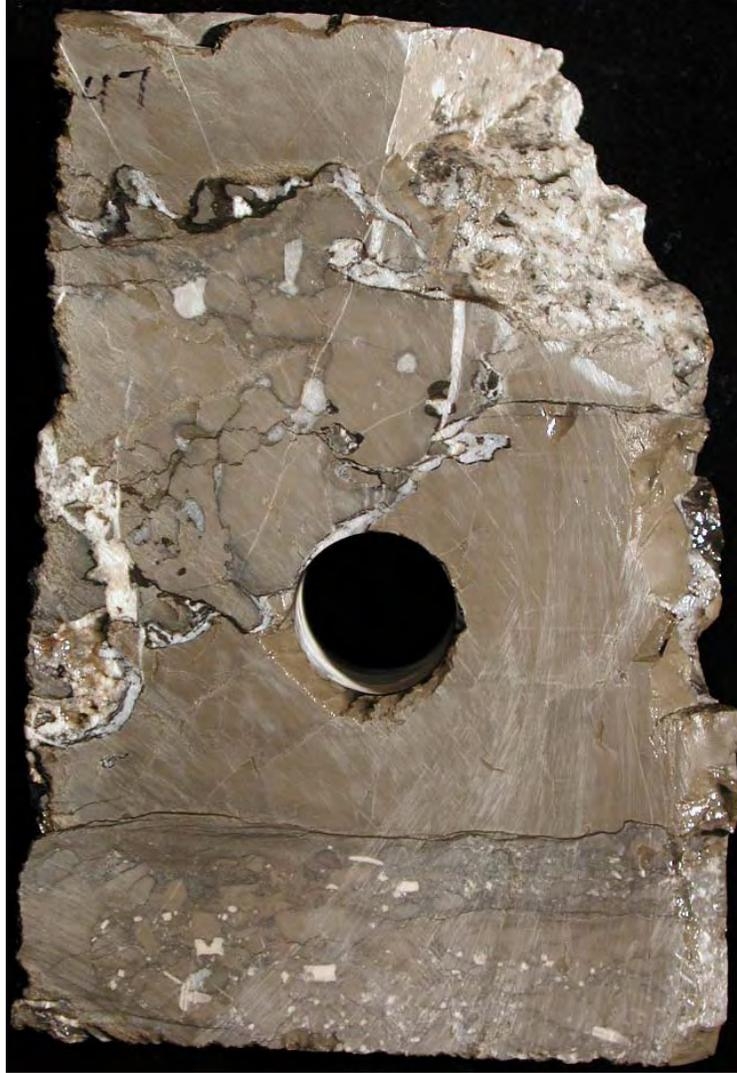
*Figure 4-5. Twin Creek Limestone reservoir rock, Watton Canyon Member, from the UPRR No. 3-3 well (section 3, T. 2 N., R. 7 E., SLBL&M, slabbed core from 8747 feet) showing highly fractured carbonate mudstone with open, bitumen-lined and calcite-filled fractures. Note zone of fossil hash at the base of the core.*
