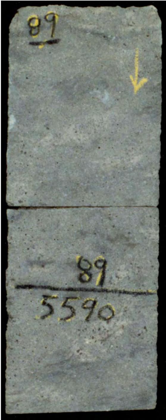
*Figure 10-27. Typical Desert Creek-zone dolomitized grainstone, calcarenite lithofacies; North Heron No. 35-C well (section 35, T. 41 S., R. 25 E., SLBL&M), Heron field, San Juan County, Utah, slabbed core from 5589 feet.*
