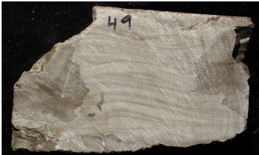
*Figure 4-3. Typical Twin Creek Limestone, Watton Canyon Member, from the UPRR No. 3-3 well (section 3, T. 2 N., R. 7 E., SLBL&M, slabbed core from 8749 feet) showing finely laminated, carbonate mudstone deposited in backbank, low-energy brackish water environment. Note that essentially no porosity is present.*
