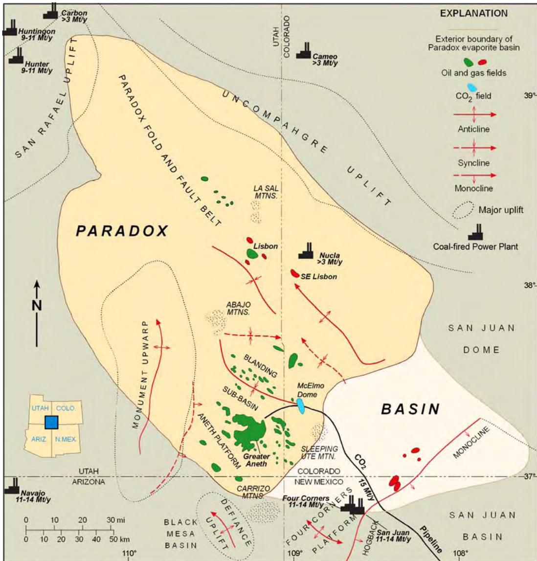
**Figure 15-23.** The locations of and emissions from surrounding coal-fired power plants (Mt/y = million tons of CO<sub>2</sub> per year), and oil and gas fields in the Paradox Basin of Utah, Colorado, and Arizona (modified from Harr, 1996). Colored (light orange) area shows present and potential of play area in the Paradox Basin.
