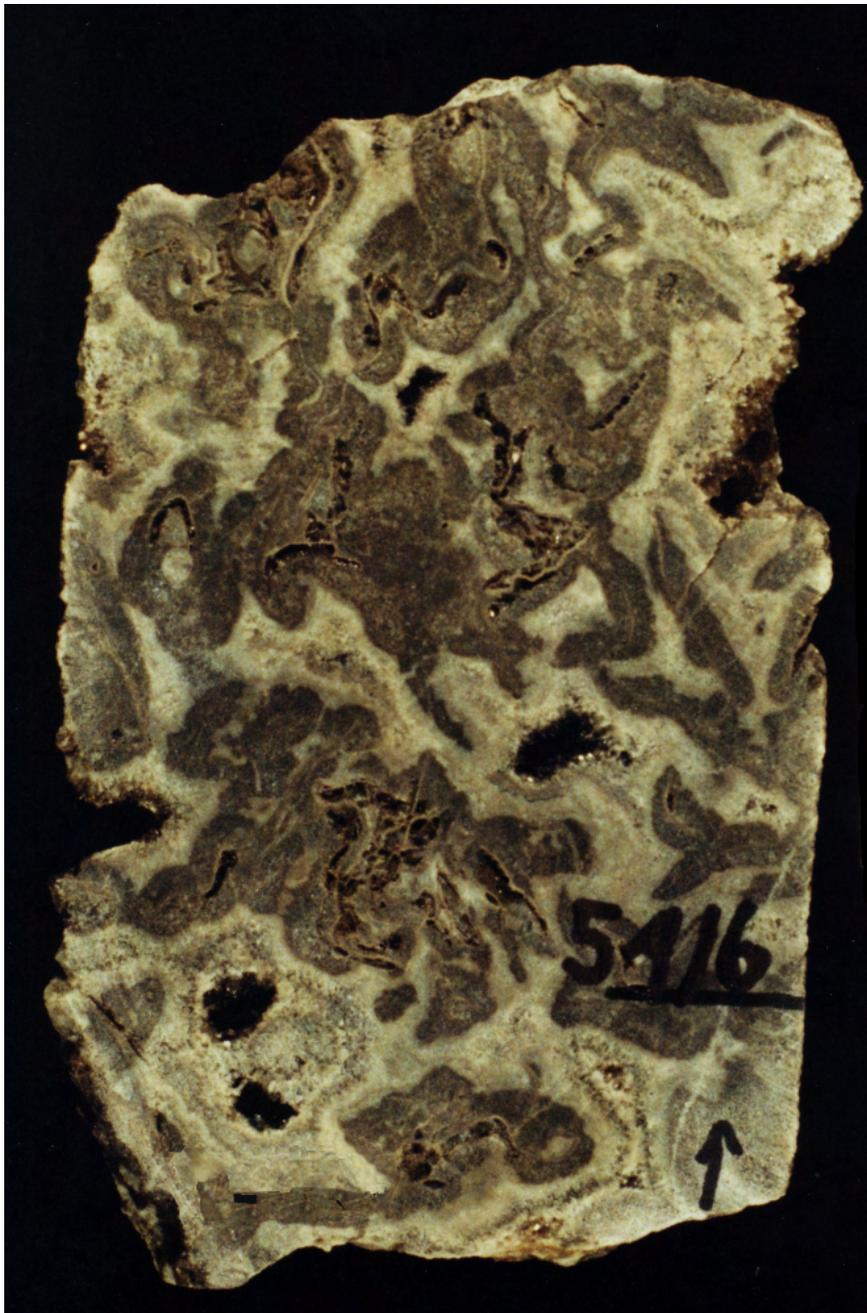
*Figure 10-44. Typical pattern of marine cementation within the well-lithified Desert Creek zone "wall" complex. Blue Hogan No. 1-J-1 well (section 1, T. 42 S., R. 23 E., SLBL&M), slabbed core from 5415.5 to 5416.1 feet, Desert Creek field, San Juan County, Utah.*
