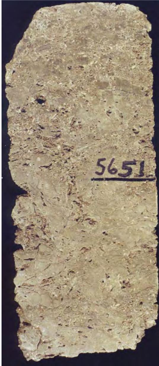
*Figure 10-29. Typical highly productive Desert Creek-zone phylloid-algal plate bafflestone; Anasazi No. 1 well (section 5, T. 42 S., R. 24 E., SLBL&M), Greater Aneth field, San Juan County, Utah, slabbed core from 5651 feet. Note good visual shelter porosity.*
