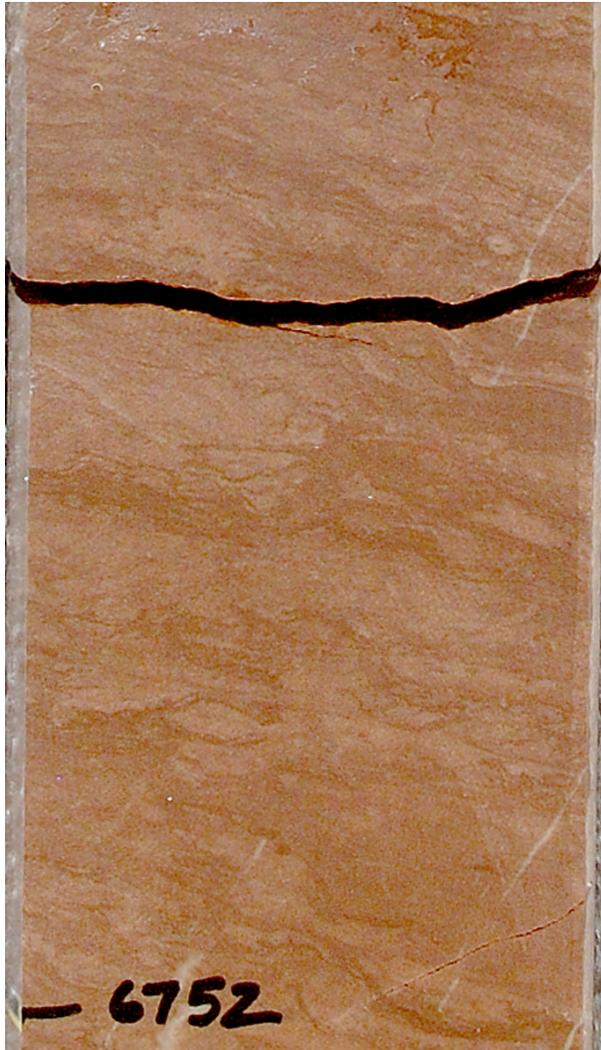
*Figure 5-8. Typical middle unit of the Navajo Sandstone, from the Kings Meadow Ranches No. 17-3 well (slabbed core from 6752 feet), Covenant field, showing siltstone laminae and shale deposited in an interdune environment.*
