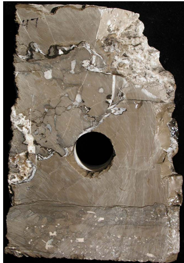
Figure 6. Twin Creek Limestone reservoir rock, Watton Canyon Member, from the UPRR No. 3-3 well (section 3, T. 2 N., R. 7 E., SLBL, slabbed core from 8747 feet) showing highly fractured carbonate mudstone with open, bitumen-lined and calcite-filled fractures. Note zone of fossil hash at the base of the core.
