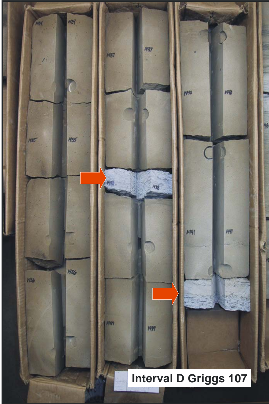
Figure 65. Cypress D interval in the Griggs 107 well in the pilot area. This homogeneous, slightly mottled, fine-grained, clean sandstone is a less common facies within the Cypress intervals yet it displays the best porosity, 21 % and permeability, 320 millidarcies. The typical wispy shale laminations were likely destroyed by burrowers. Thin, ripple laminated sandstone beds with flat rip-up clasts at 1438 and 1441 feet are probably the result of changes in depositional energy or sediment supply and, if extensive, can compartmentalize this interval.
