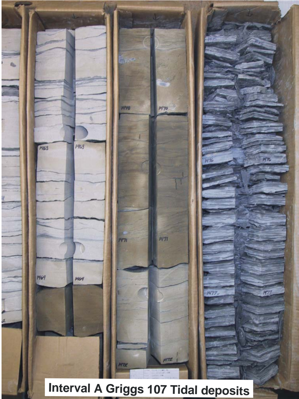
Figure 69. Core from Plains Illinois Griggs 107 well Sec. 32-T4N-R12W. Contact between oil stained reservoir quality sandstone with high core measured porosity and permeability values and interbedded, flaser bedded siltstone and shale permeability barrier.
