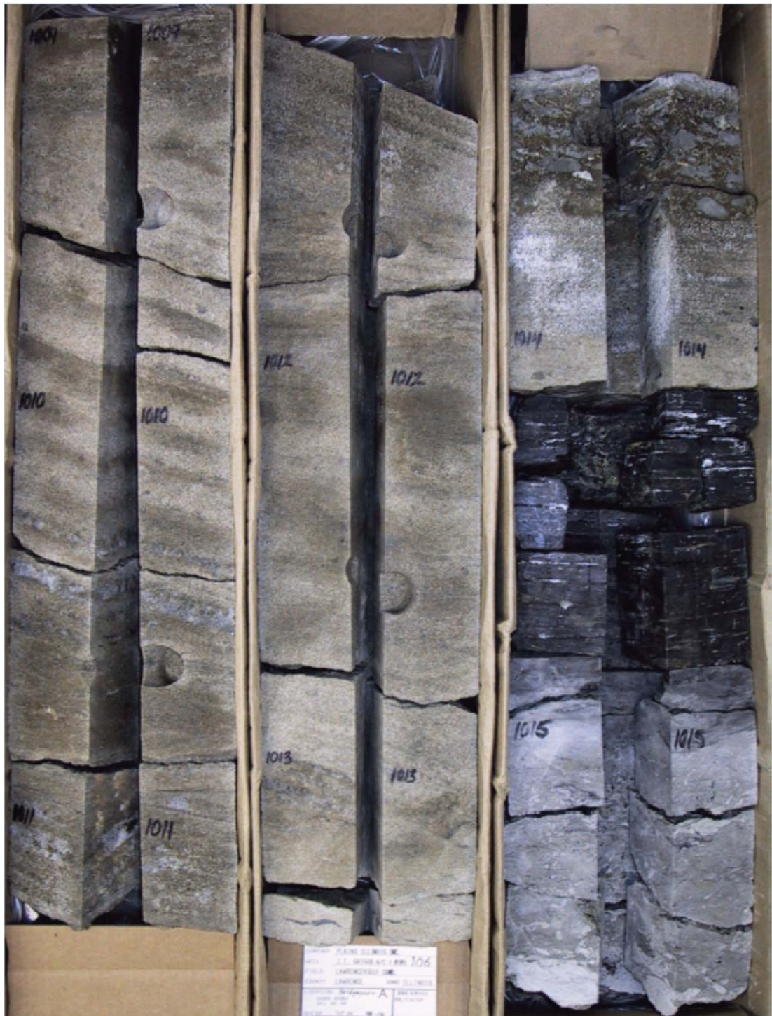
Figure 17. Core example of the Bridgeport A channel characteristics from the Griggs #106 well in the Se Ne of section 32. Medium to high angle tabular cross-bedded sandstones with pyrite cement is very common in the Bridgeport A sandstones particularly in the basal cross-beds, and occurs as banding and nodules in these beds. This channel scoured into a peat bog at its base. The banded oil staining in the core shows the influence of the cyclical cementation and reduction in reservoir quality.
