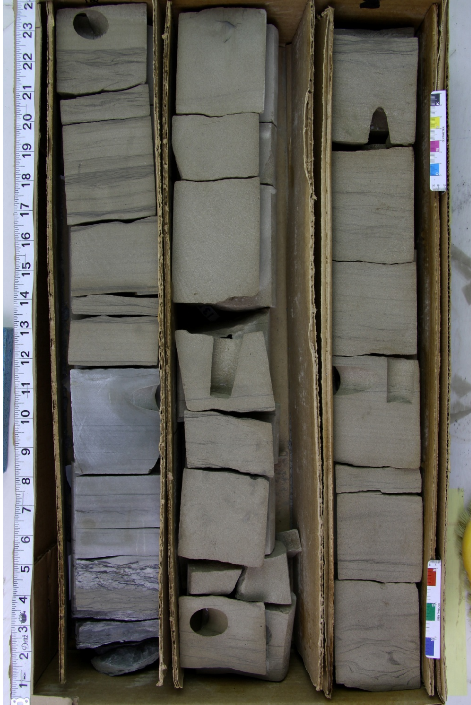
Figure 67. 121012892800 1307'-1313.5' Parallel tidal rhythmites and tidal couplets. Calcite cemented sandstone interval are present in the continuation of cored Cypress Sandstone interval from previous figure
