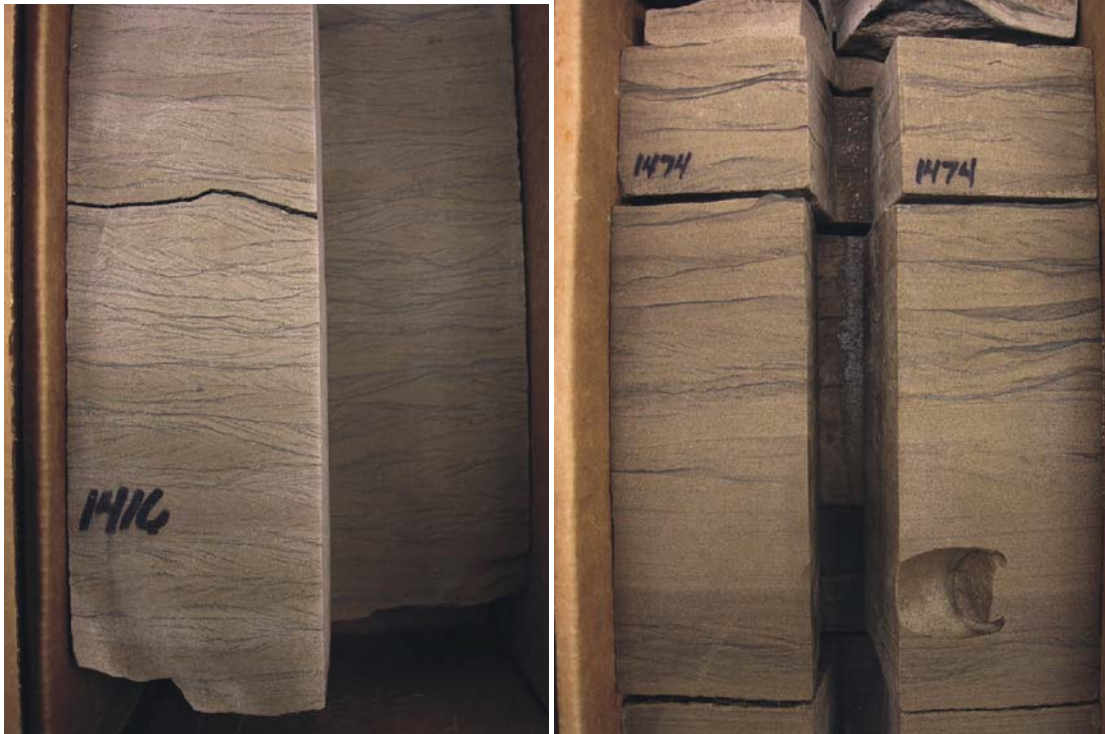
Figure 68. Griggs 106 well. .Left example from the Cypress E Interval of herringbone and reverse bedded, ripple cross-laminated reservoir sandstone. Dark wispy, wavy clay laminations are ubiquitous within this facies. This is the predominant reservoir facies within all the Cypress intervals in this and nearby areas of study. Slight variations of this facies include subparallel-to horizontal laminated sandstone with a decrease in the pencil-thin, dark gray clay laminations. Herringbone bedding is indicative of tidal current influence on these sediments which are tentatively interpreted as tidal shoal or bar deposits.
