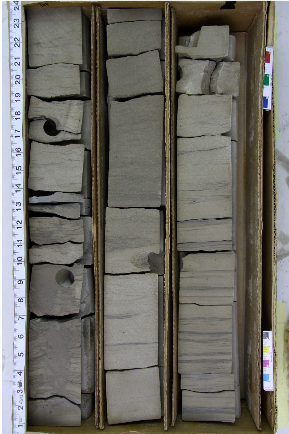
Figure 66. 121012892800 1301'-1307'. Very fine grained sandstone, tidal deposits. Escape burrow through several alternating fine and very fine grained episodes of sedimentation at 3002'. Tidal laminations and rhythmites can be viewed at 1307.
