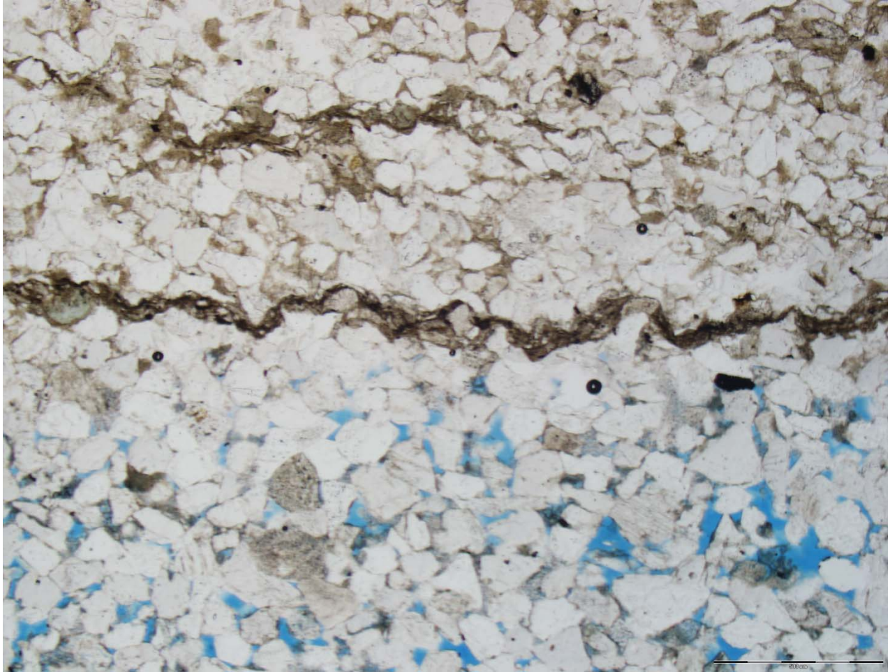
Figure 82. Example from the Griggs 107 at 1453.4' shows porous laminae alternating with non-porous laminae. Porosity is highlighted by medium blue stained epoxy. A stylolitic parting separates the nonporous tightly cemented fine-grained sandstone from the porous sandstone.
