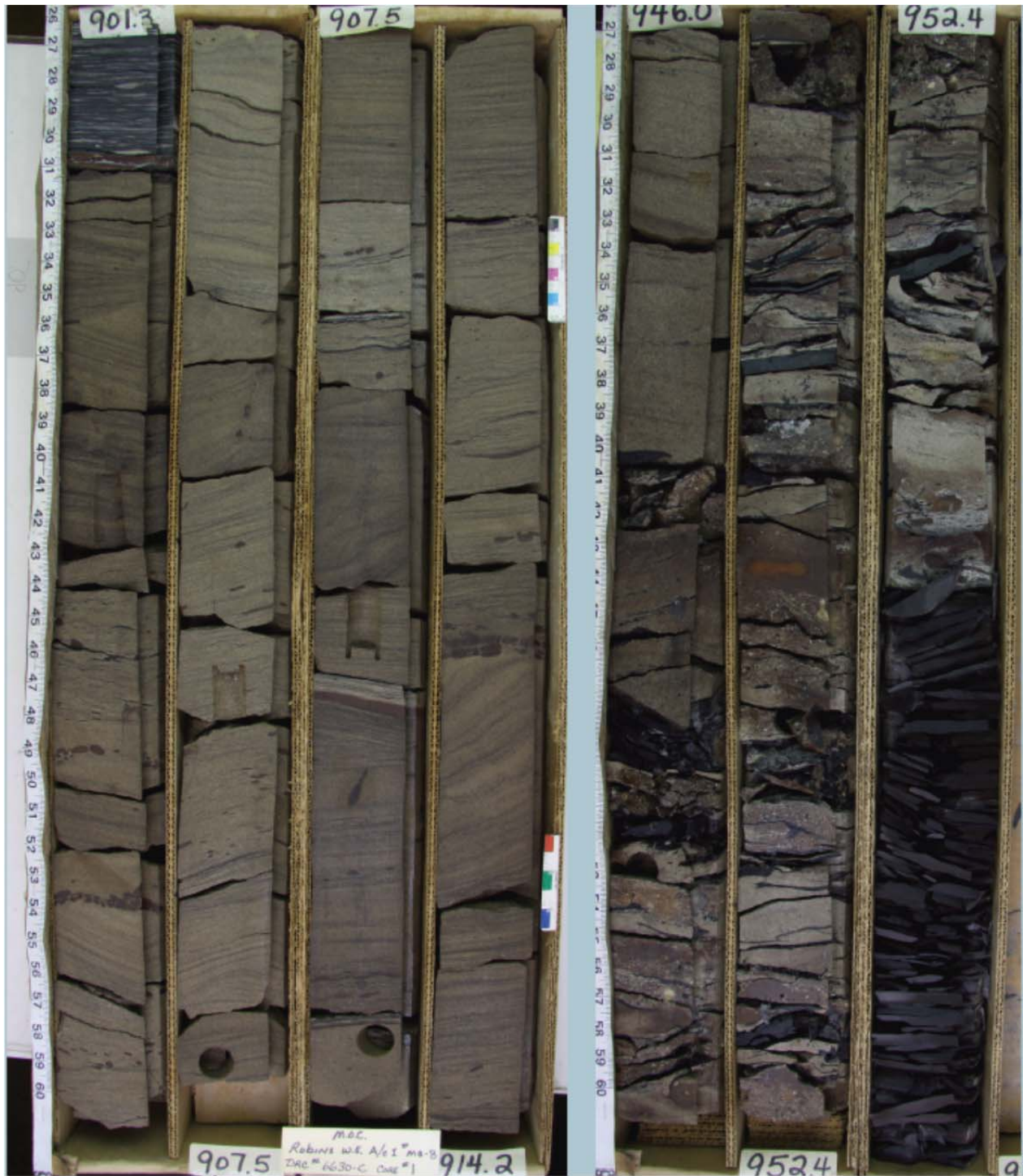
Figure 35. Core example of channel fill Bridgeport B stratigraphic equivalent from the Robbins MG #8 well near the Maraflood pilot in section 5. Sharp scour contact with course rip-up and conglomeratic basal channel lag (approx. 950- 958 feet) transitions into very clean tabular cross bedded sandstone throughout most of the channel facies. Some core shows possible marine indicators in the upper feet of the core (tidal couplets and trace fossils).
