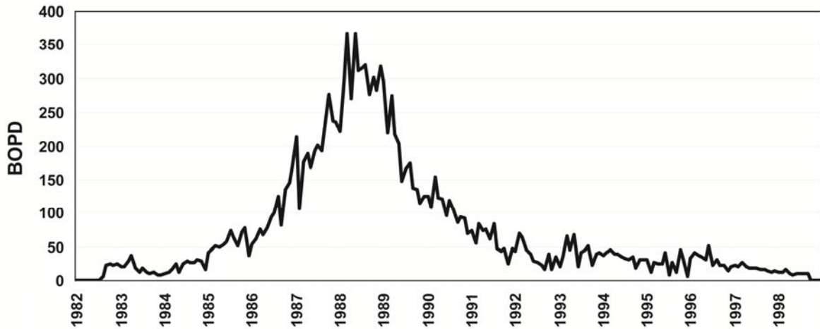
Figure 4. Graph showing increased production from the Robins 102-B Maraflood surfactant flood starting in 1982. The 25 acre Bridgeport B channel sandstone pilot project in the SE quarter of Section 5, T3N R12W achieved 34% SOR recovery (15% PV), 450 mbo. The flood was a scientific success but was not expanded. An oil price drop at this time apparently did not offset the cost of polymer and surfactant.
