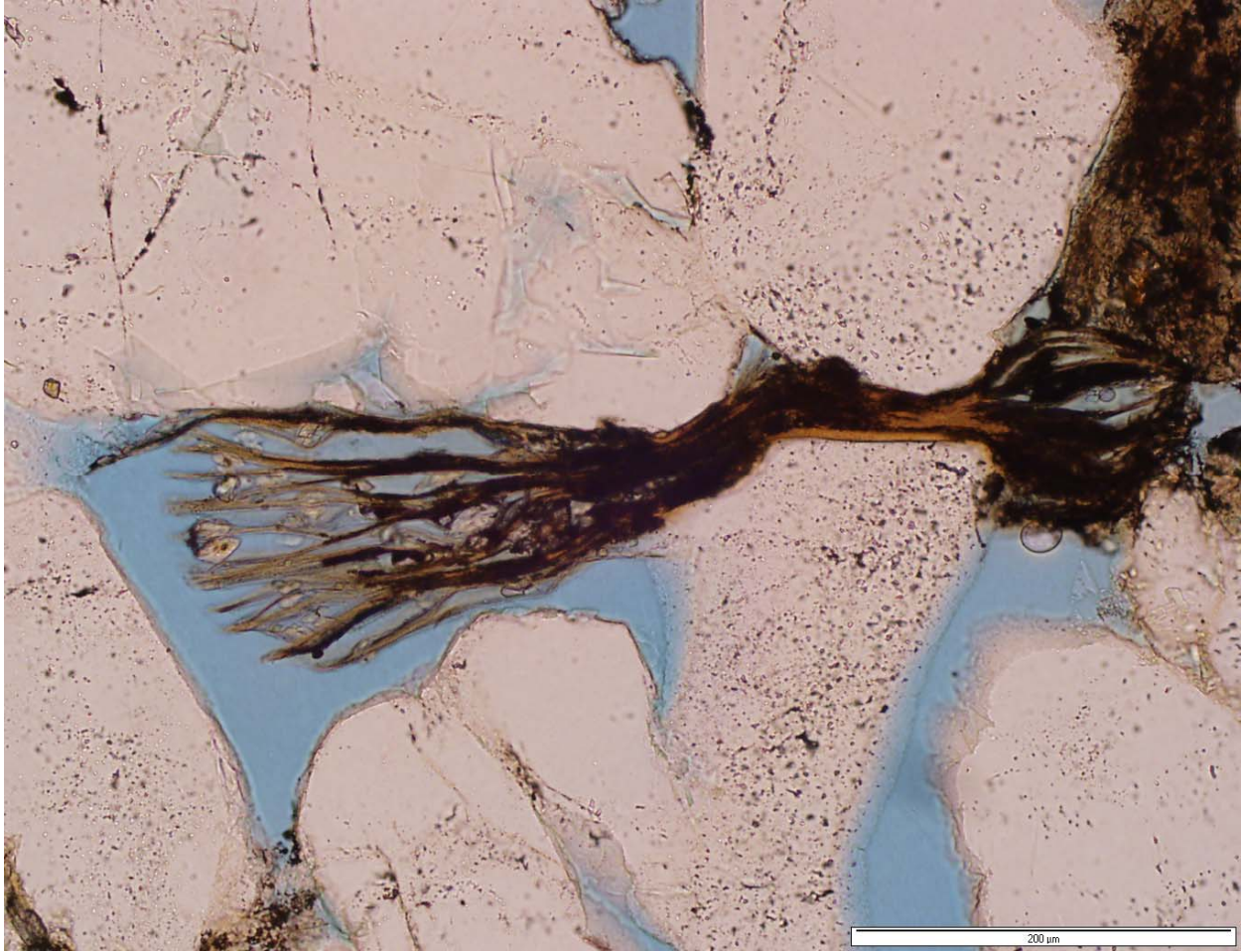
Figure 45. Thin section from 121012871800 Robins ME-10 well depth 953.4 ft., 20X white transmitted light, horizontal permeability is 557md, vertical permeability is 178md, and porosity is 22.3%.
