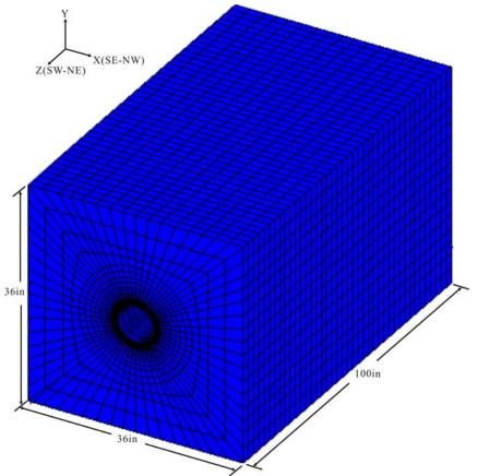
Figure 9-17. Model for the horizontal well parallel/perpendicular to the maximum horizontal principal stress,  $\sigma_{\rm H}$ .
