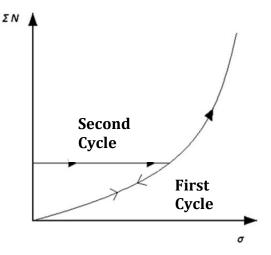
Figure 10-2. A graph of the cumulative AE hits ( $\Sigma$  N) versus stress ( $\sigma$ ) for two loading cycles subject to uniaxial compression.
