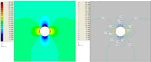
Figure 9-28. Case 2: The minimum principal stress  $\sigma_3$  around the well bore section.
