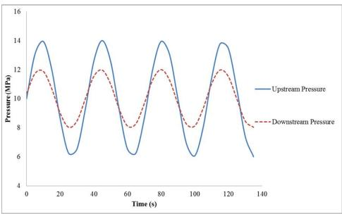
Figure 7-7 Changes of the pressure during a sinusoidal oscillation pulse method
