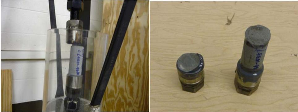
Figure 8-3 Pictures of the destruction of core plug after tensile strength test.
