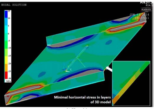
(b) 3D model Figure 5-29a. Contour map of minimum horizontal stress.
