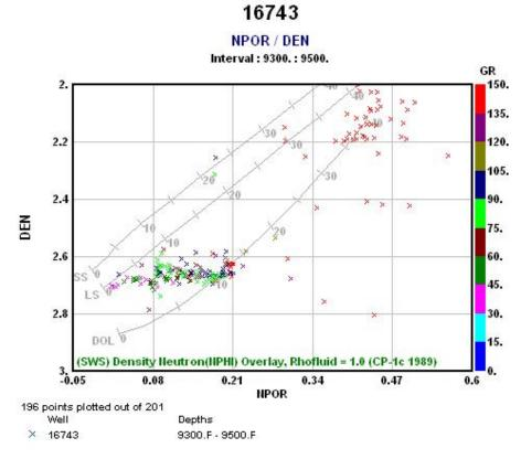
Figure 3-7: Neutron/density cross plot of Well#16743
