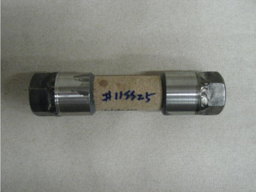
Figure 7-24. Specimen glued to steel caps
