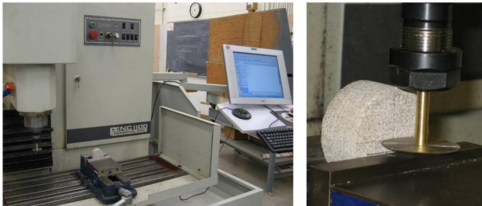
Figure 10-22. CCNBD specimen preparation
