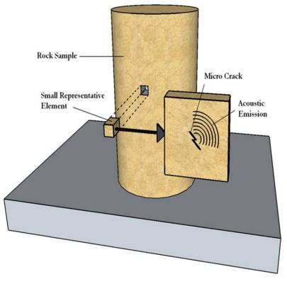
Figure 10-5. The microcrack model for AE
