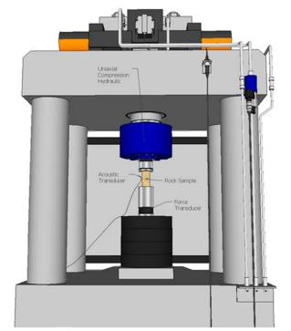
Figure 10-7. A close-up picture of the Uniaxial Loading Method (816 Rock Test System)
