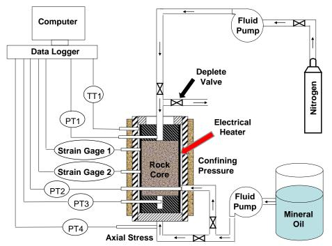
Figure 7-3 Experimental setup for permeability measurement under stresses
