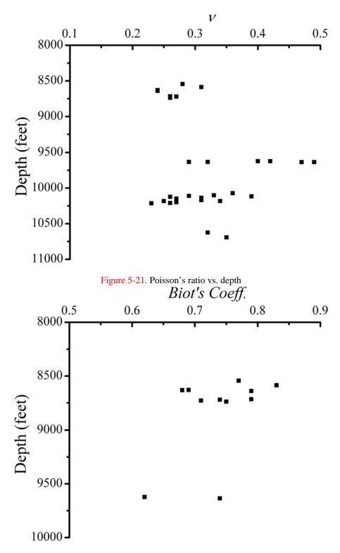
Figure 5-22. Biot's coefficient vs. depth
