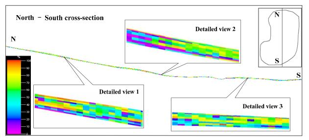
Figure 4-15. North-South cross-section view, 5cm based RQD index
