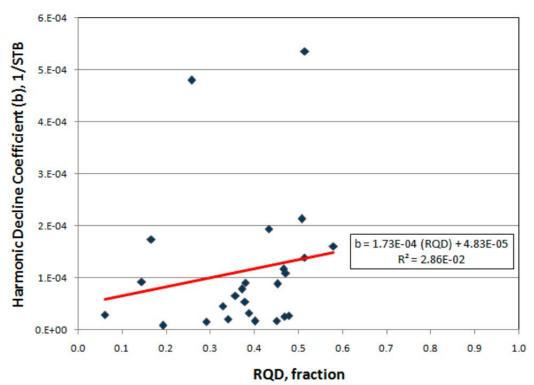
Figure 4-30. Decline coefficients of wells vs. RQD
