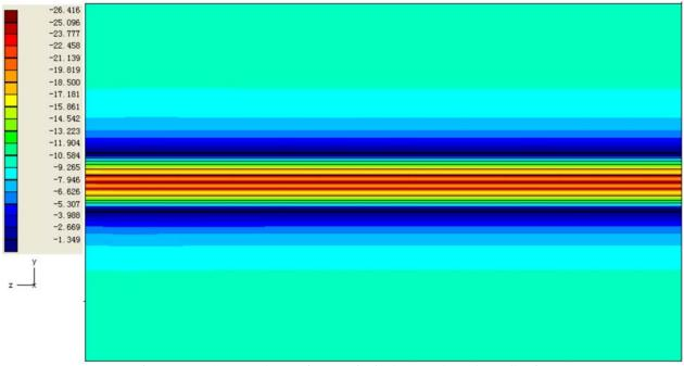
Figure 9-29. Case 2: The maximum principal stress along the well axis.
