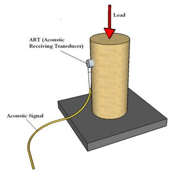
Figure 10-6. Rock sample showing direction of vertical stress and attachment of ART's (Acoustic Receiving Transducers)
