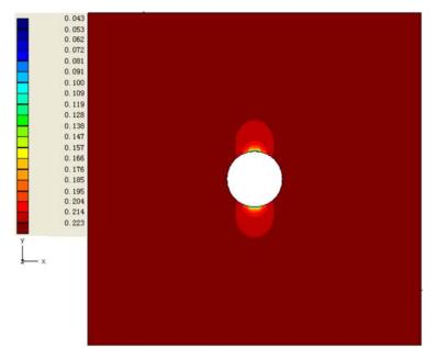
Figure 9-31. Case 2: Safety coefficient for minimum principal stresses. Possible tensile failure on top and bottom of the well bore.
