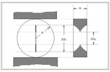
Figure 10-21. The cracked chevron notched Brazilian disc specimen (modified after ISRM, 1995)
