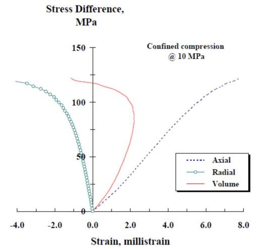
Figure 7-20. Strain and stress data collected on a sample
