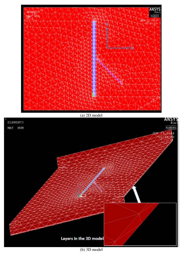
Figure 5-28. Different materials used for the elements: cyan (Material 1) – fault core, purple (Material 2) – damage zone, and red (Material 3) – host rock.
