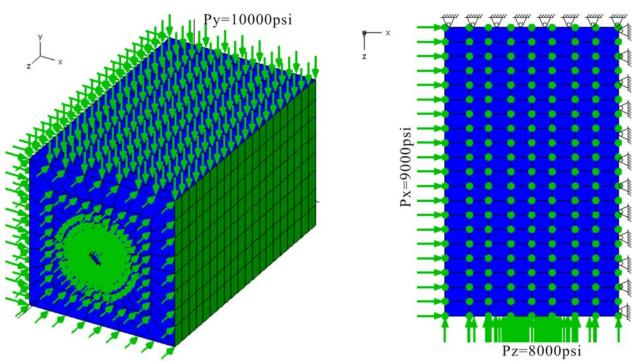
Figure 9-20. Boundary conditions for the Case 2, well axis perpendicular to  $\sigma_{H}$ .
