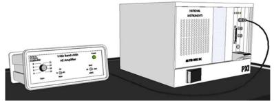
Figure 10-10. Wide band width amplifier (left) and NI Chassis (right) with a high-resolution digitizer and interface card installed.
