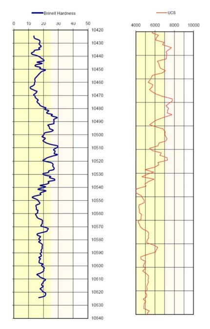
Figure 5-14. UCS and Brinell hardness curve in Well WT1(NDIC, 2007a)
