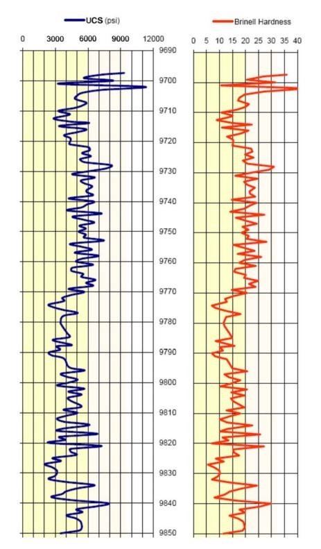
Figure 5-16. UCS and Brinell hardness curve in well WT3 (NDIC, 2007b)
