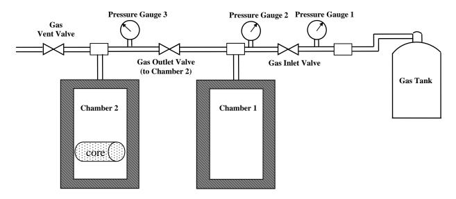
Figure 7-6. Schematic of facility to measure rock porosity
