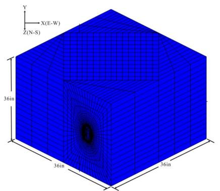
Figure 9-18. Model for a horizontal well at 45° angle to the maximum horizontal principal stress,  $\sigma_{\rm H}$ .
