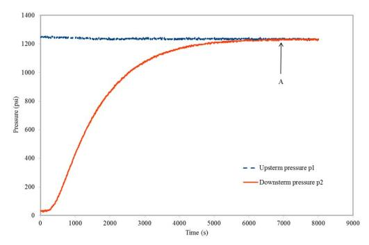
Figure 7-11 Changes of the downstream pressures while maintaining constant upstream pressure The upstream pressure  $(p_1)$  is constant, and the downstream pressure  $(p_2)$  builds up through the time.
