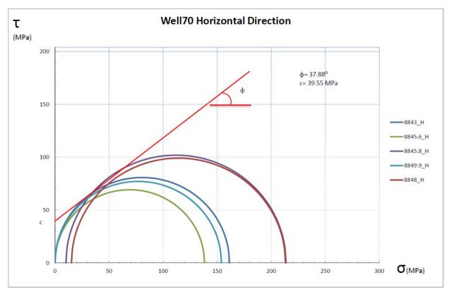
Figure 7-21 Mohr envelop for Bakken formation, established by drawing the best fit tangent to experimentally determined failure stresses at a range of confining pressures and isothermal conditions
