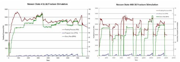
Figure 6-1. Pump plot of the hydraulic stimulation test (after Headington Oil LLC and XTO Energy Inc, 2008).
