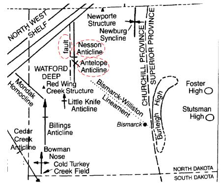
Figure 5-1. Major structural features of the Williston basin, North Dakota portion (After Gerhard et al., 1990).
