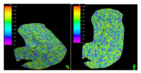
Figure 4-8. The RQD index (10 cm based) in middle Bakken Formation green arrow pointing to north
