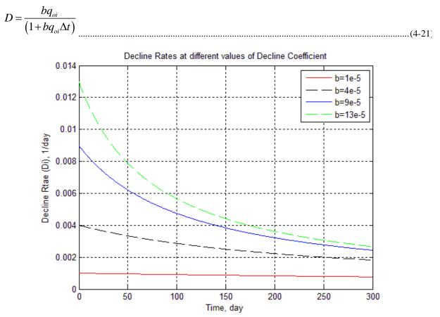
Figure 4-29. Effect of Decline coefficient on decline rate
