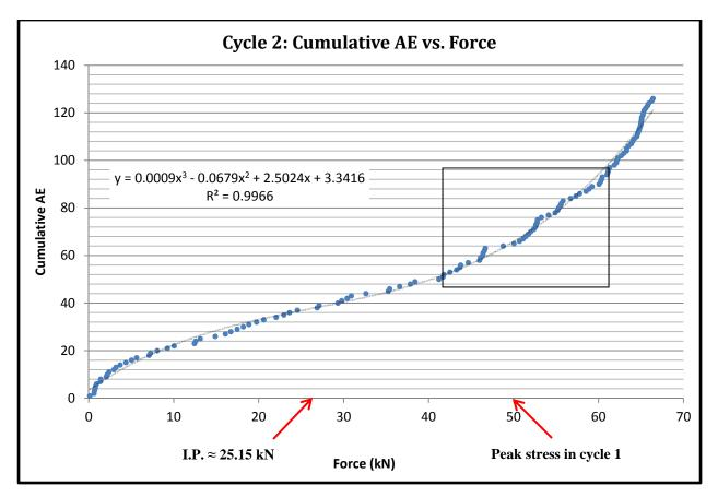
Figure 10-20. Cumulative AE for 126 acoustic events gathered over a time of 22.78 minutes in cycle 2
