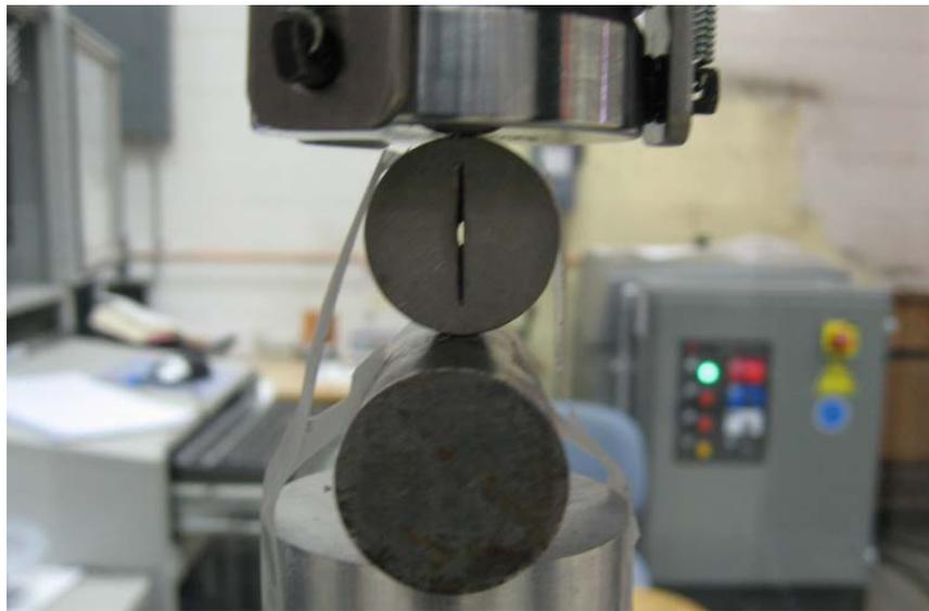
Figure 10-29. Shale sample under compression at MTS station
