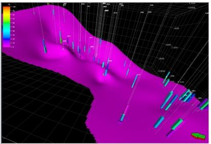
Figure 4-5. 3D geological model with the RQD index along the corresponding well path in Petrel
