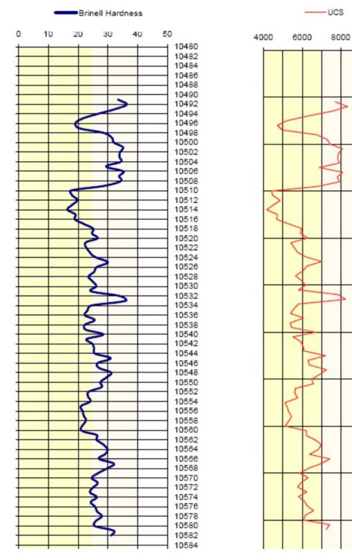
Figure 5-15. UCS and Brinell hardness curve in Well WT2 (NDIC, 2006)
