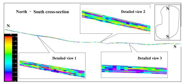
Figure 4-10. North-South cross-section view, 10 cm based RQD index
