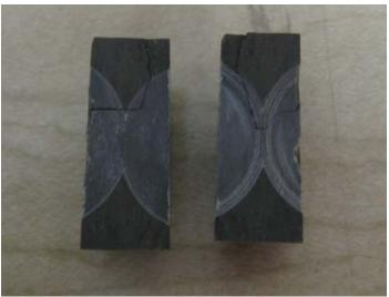
Figure 10-30. Fractured surface after tests
