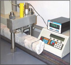
Figure 5-12. Brinell Hardness Test Apparatus. (UCS as determined from Brinell Hardness using slabbed core sections)
