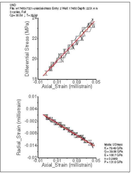
Figure 7-18 An example of stress and strain in a non-destructive strength test in this study
