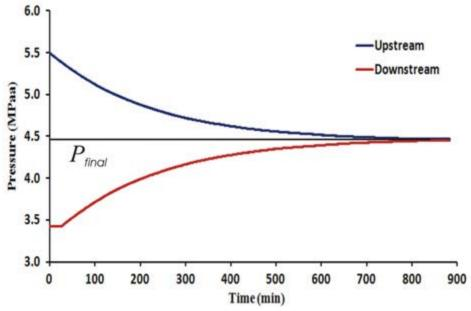
Figure 7-9 Changes of upstream and downstream pressures in pulse decay method
