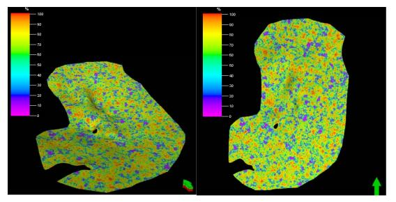
Figure 4-13. The RQD index (5cm based) in middle Bakken Formation, green arrow pointing to north
