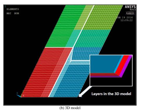
Figure 6-4. Different materials used for the elements. Different colors represent different materials in the model.
