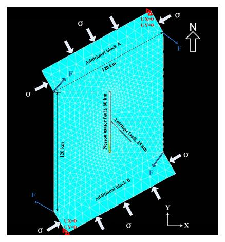
Figure 5-27. Plan view from Z (vertical) direction of the finite element model.
