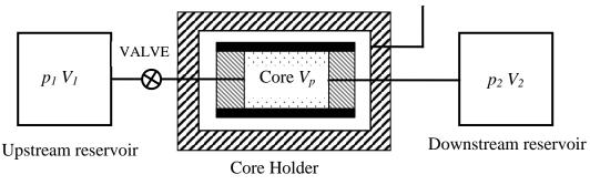
Figure 7-8 Schematic diagram for pulse decay permeability system
