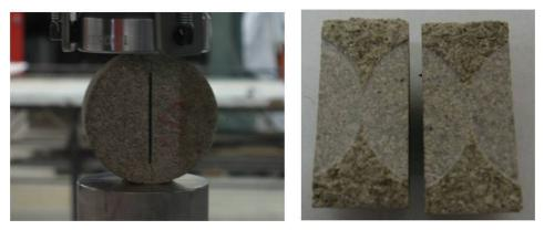
Figure 10-23. Sample compressed by MTS rock tester and the fracture surface after failure
