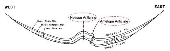
Figure 5-2. Cross section view of the Nesson anticline and Antelope anticline (after Meissner, 1978).
