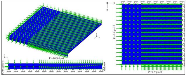
Figure 9-10. Boundary conditions for the numerical model.
