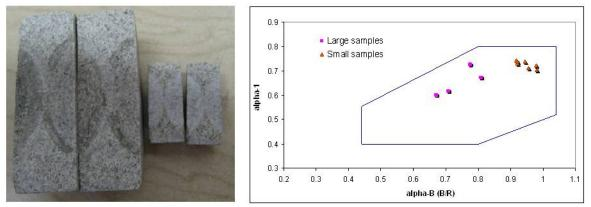
Figure 10-25. Both large and small samples (left) are in the valid geometrical range (right).
