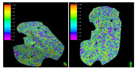
Figure 4-14. The RQD index (5cm based) in lower Bakken Formation, green arrow pointing to north
