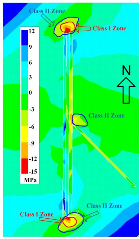
Figure 5-31. Possible zones for natural tensile fracture development.
