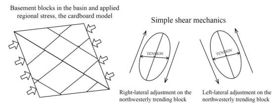
Figure 5-8. Regional stress applied on the basement blocks during the Laramide orogeny, and response of the northeasterly trending blocks and northwesterly trending blocks, according to the simple shear model (After Thomas, 1974).
