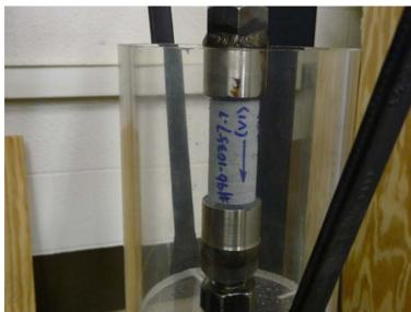
Figure 8-2 The installation of core plug on tensile strength test apparatus.
