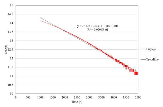
Figure 7-10  $\ln(\Delta p)$  vs. time plot for core sample permeability measurement using pulse decay method
