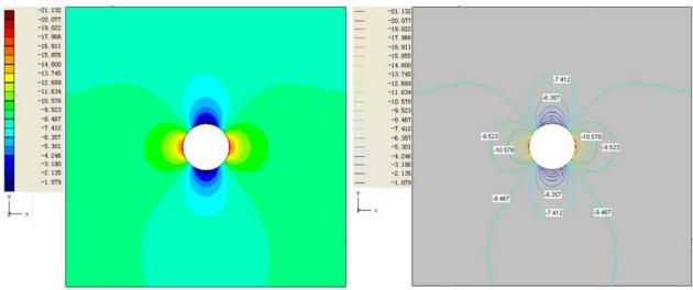
Figure 9-27. Case 2: The maximum principal stress  $\sigma_1$  around the well bore section.
