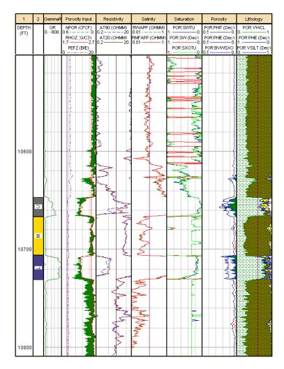
Figure 3-8: Well logs interpretation results: lithology, porosity, and saturation
