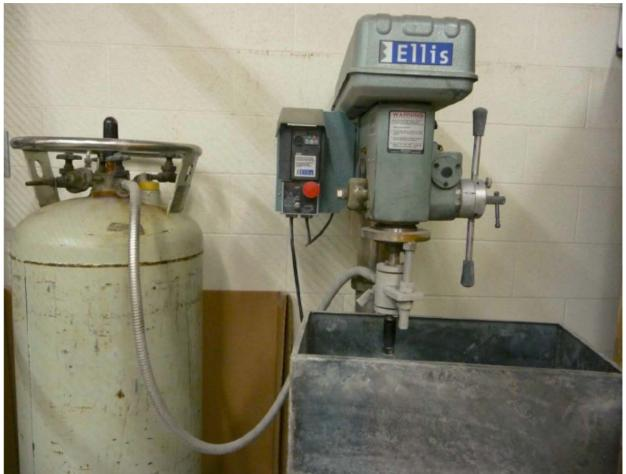
Figure 7-1 Core plug sampling system used in this study
