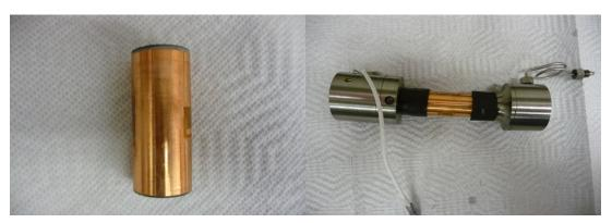
Figure 7-4 Images of core and core holder for rock properties test
