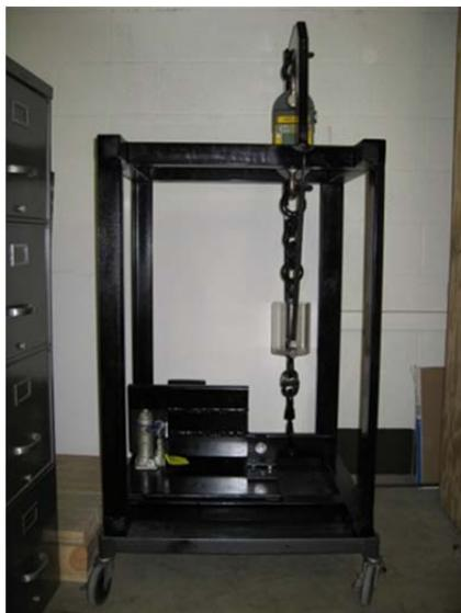
Figure 7-22. Tensile strength test apparatus
