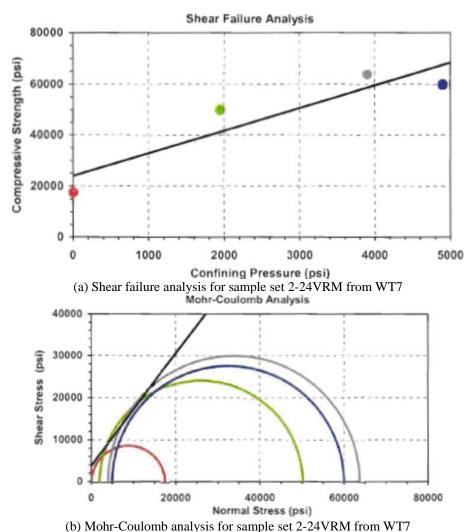
Figure 5-18. Shear and Mohr-Coulomb analysis for sample set 2-24VRM from WT7 (NDIC, 2010)
