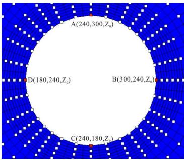
Figure 9-35. Stress monitoring points around the well section.
