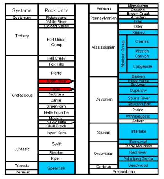
Figure 1-2. Generalized stratigraphic column for Williston basin with the oil producing horizons in blue and the two gas producing horizons in red (Heck et al, 2002).
