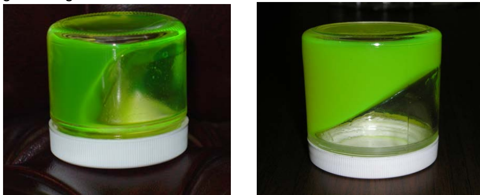
Figures 1-A & B. Low to Medium Concentration SPI Gel Samples. A-internal initiator; B-CO 2 external initiator.
