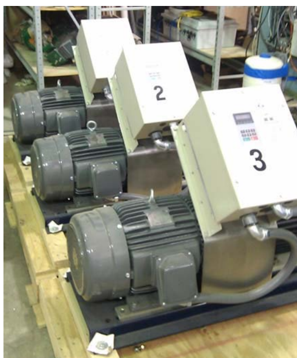
Figure 13. Three Hydra-Cell Diaphragm-type (positive displacement) Chemical Metering pumps with Variable Speed Controllers
