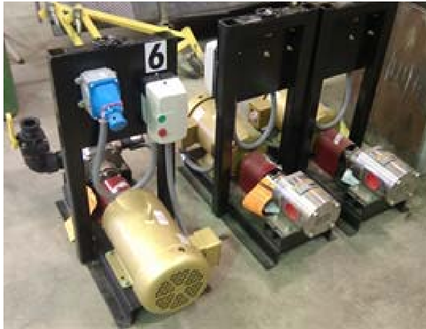
Figure 14. Stainless Steel and Polyethylene low pressure, high rate gear-type transfer pumps - electric powered. Not shown-gas powered Polyethylene gear pump.
