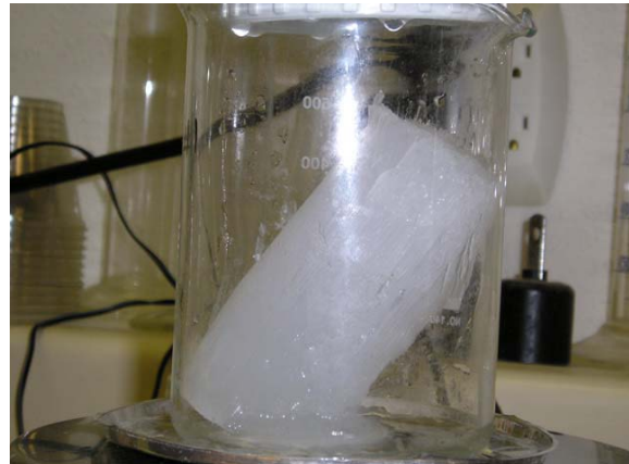
Figure 7. SPI Gel through BGST and partially reformed into a block
