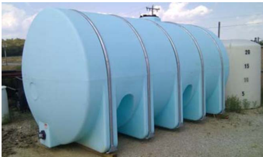
Figure 12. Four 5025 gallon (120 bbls) Norwesco Polyethylene Chemical Storage Tanks (blue front) w/steel base skid added later. White 25 bbl polycarbonate water tank.
