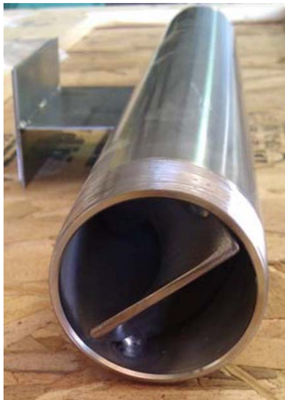
Figure 11. UET In-Line Stainless Steel Internal Static Mixer rated for 2700+ psi and 3000 BPD, installed on the Mixing Skid.
