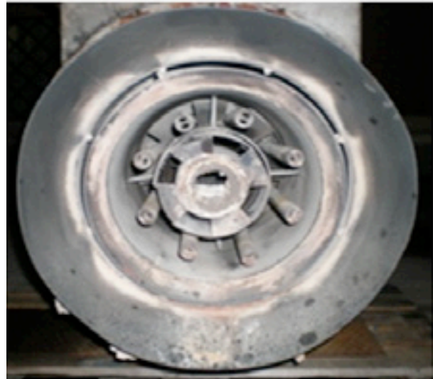
Figure 2. (left) Computational domain developed for the TEA-C burner in STAR-CCM+. (right) Photograph showing actual TEA-C burner.
