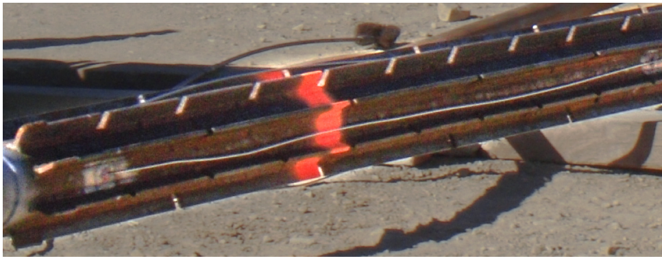
Figure 5. Heater used small experimental tests at the AMSO site.
