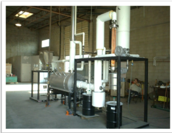
Figure 1: Amaron Energy 1/2 ton/day prototype pyrolysis kiln.
