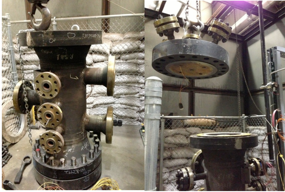
Figure 12. (left) Body of the pressure vessel. The flanges seen have been fitted with “feedthroughs” to extract cables for thermocouples, linear variable differential transducers (LVDTs), and a load cell. (right) Lowering the upper closure onto the vessel.
