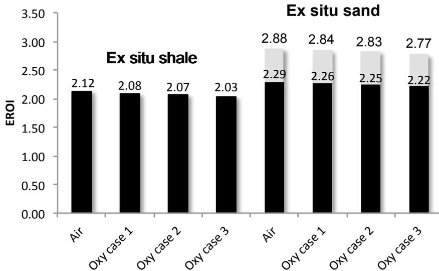
**Figure 3.** Point-of-consumption NER and net external energy return (NEER) estimates for the air-fired baseline and three oxyfired cases. For the shale cases, NER and NEER are equal, but for the sand cases NER (lower value) and NEER (higher value) are both presented. In situ sand is excluded because the baseline NER is less than one.
