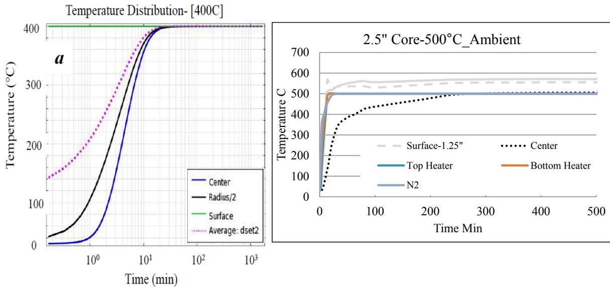
Figure 11. (left) Temperature distribution at various locations in sample from multi-physics COMSOL simulation of 10 cm diameter sample with a surface temperature of 400°C. (right) Temperature distribution from core experiment performed with a 6.35 cm diameter sample and a surface temperature of 500°C.
