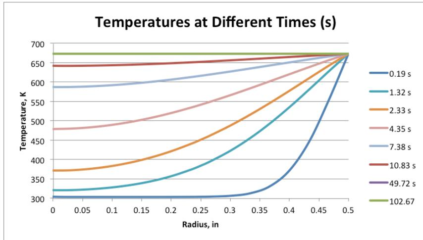
Figure 12. Temperature gradient of a core with a 2.54 cm diameter at various times.
