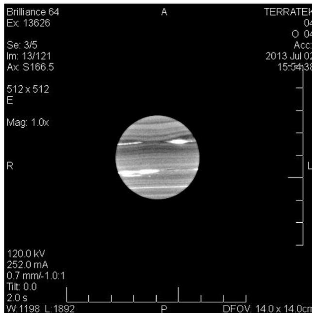
**Figure 20.** One of multiple (every mm) cross-sectional CT scans of a Skyline oil shale plug (1-inch diameter).
