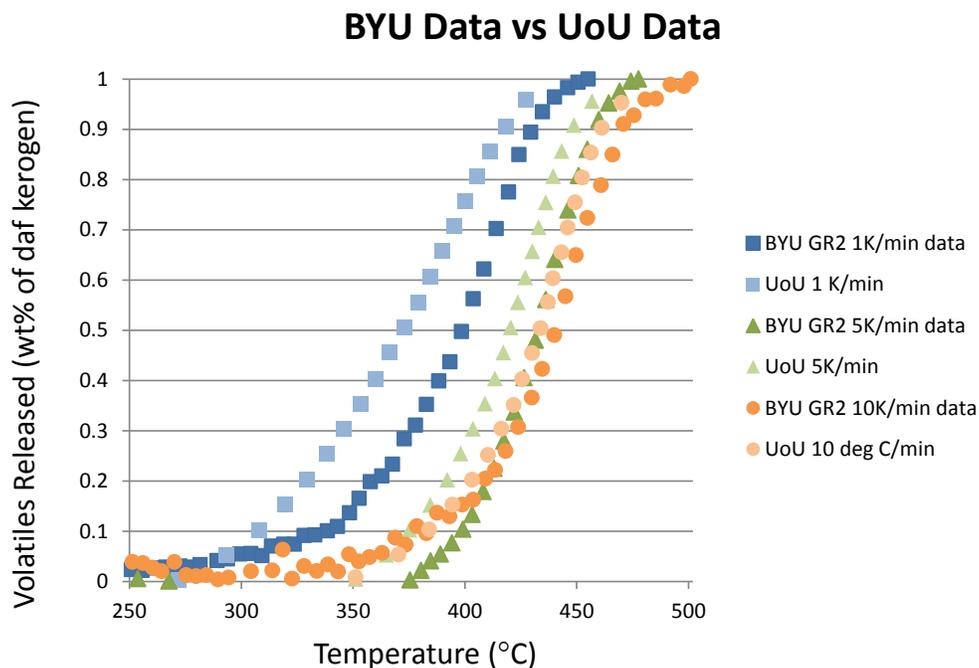
**Figure 16.** Comparison of BYU vs. UU pyrolysis data from the GR2 sample at atmospheric pressure and heating rates of 1, 5, and 10 K/min.
