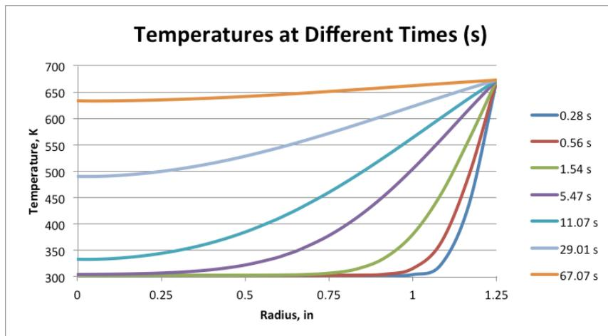
Figure 14. Temperature gradient of a core with a 6.35 cm diameter at various times.
