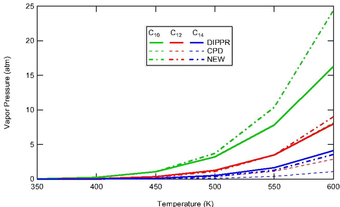
**Figure 17.** Vapor pressures computed for *n*-decane, *n*-dodecane, and *n*-tetradecane as a function of temperature. Also shown are vapor pressures computed from the CPD correlation for coal tar vapor pressures and the new correlation for *n*-alkanes.
