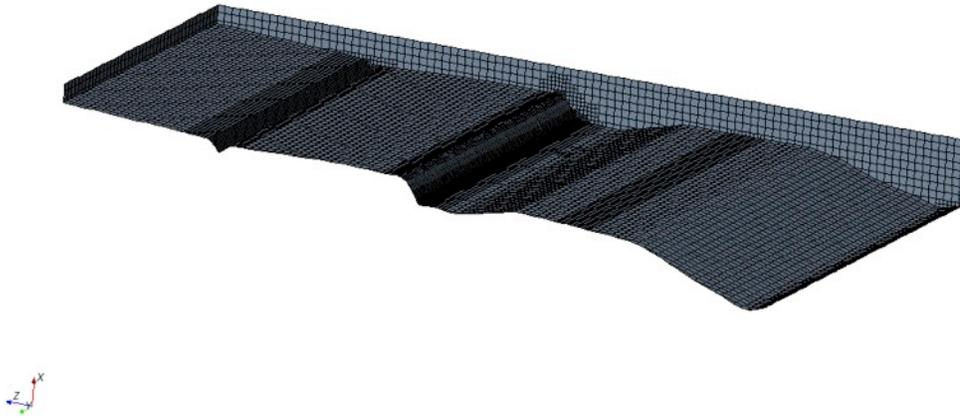
**Figure 7.** Close-up of the mesh for one piece of shale.
