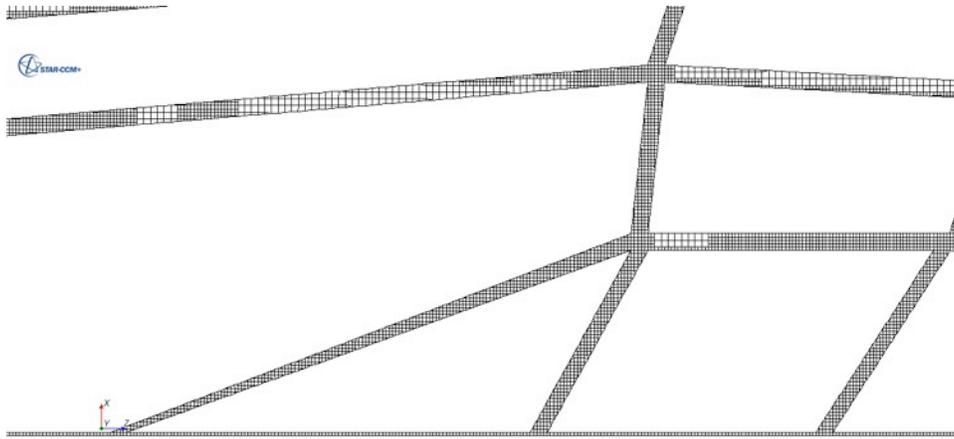
**Figure 9.** Close-up of the very fine mesh used to capture the fluid movement inside the convective channels which occur between the pieces of shale (solid white color in this figure).
