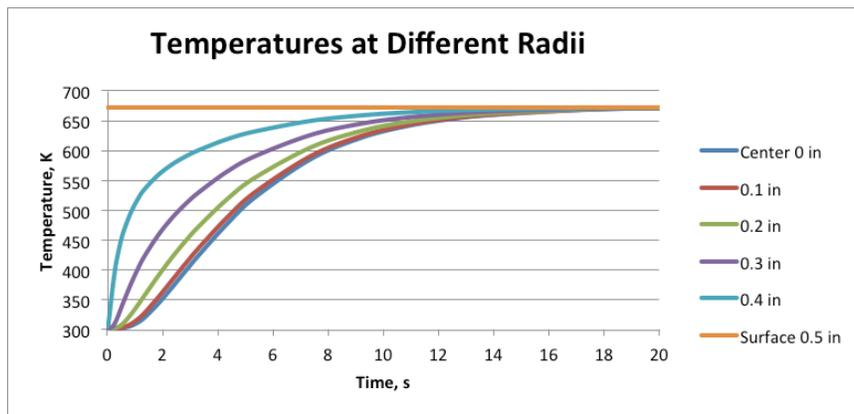
Figure 13. Temperature gradient of a core with a 2.54 cm diameter at various radii.
