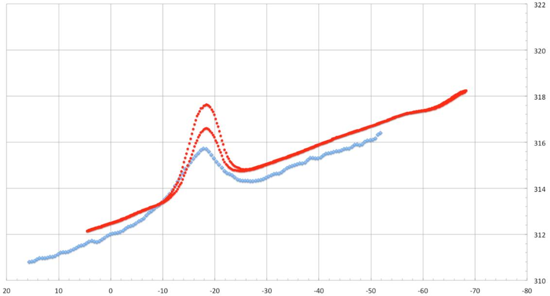
**Figure 14. Comparison of temperature distribution in one of the tomography wells for simulation (red markers) and experimental results (blue markers). Horizontal axis represents depth, while the vertical axis represents the temperature.**
