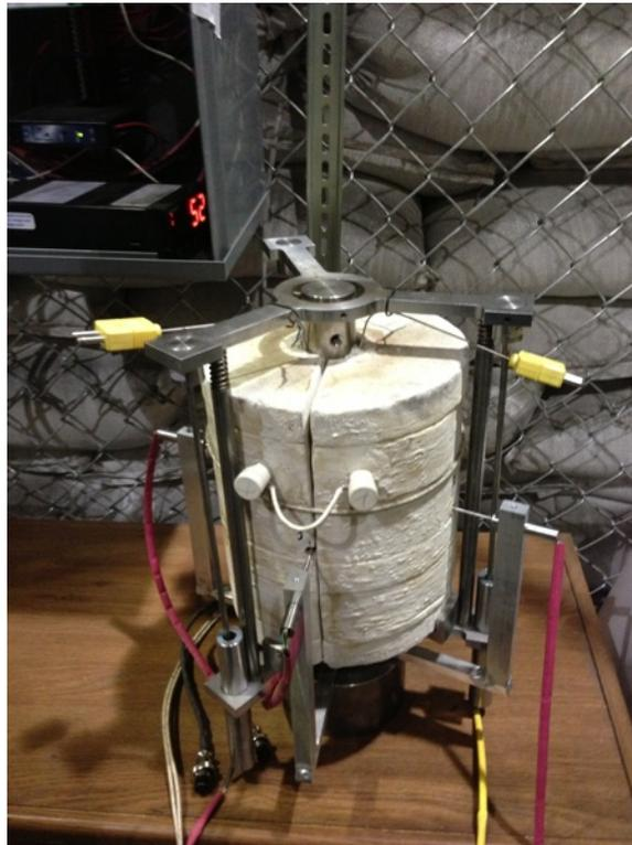
**Figure 18.** Clamshell heater with radial and axial cantilevers mounted. For scale, the heater is about 12 inches in height.
