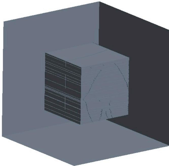
**Figure 5.** Modified simulation geometry used to study the effect of rubblization on the overall heat transfer inside the generalized shale formation.
