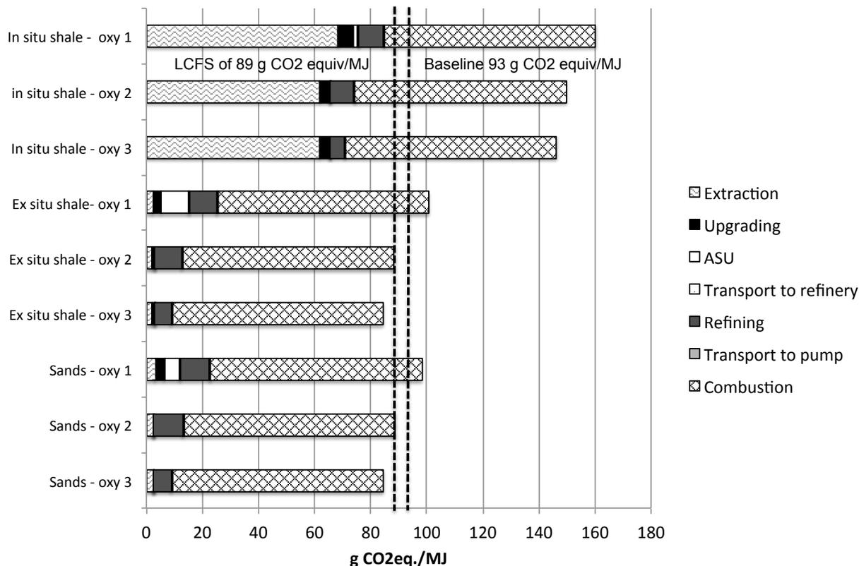
**Figure 2.** Comparison of estimated WTW GHG emissions for ex situ Utah oil sands and shale with the California LCFS of 89 g CO<sub>2</sub> e/MJ and the baseline GHG emissions associated with the Energy Independence and Security Act.
