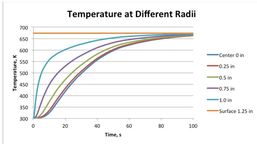
**Figure 15.** Temperature gradient of a core with a 6.35 cm diameter at various radii.
