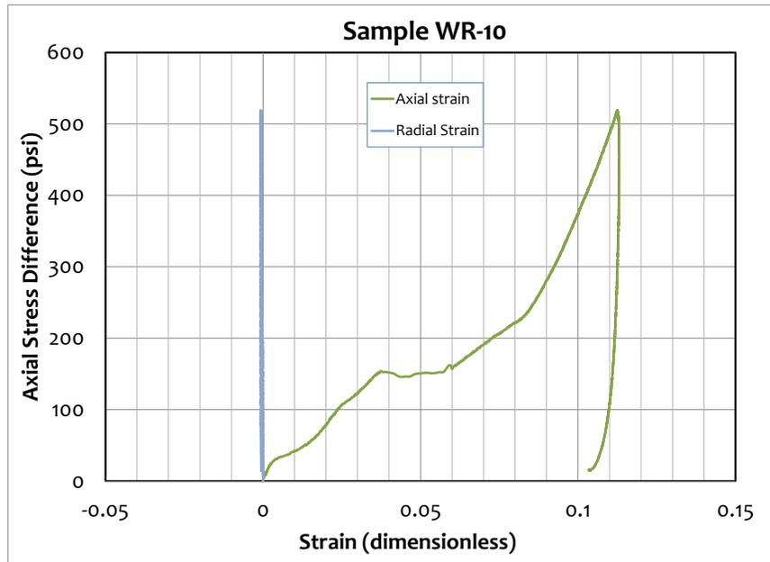
**Figure 19.** (top) Snapshot of stress, strain and temperature during a portion of a test on a White River sample. The confining pressure (1400 psi) is also shown. (bottom) Axial stress difference versus axial and radial strain.
