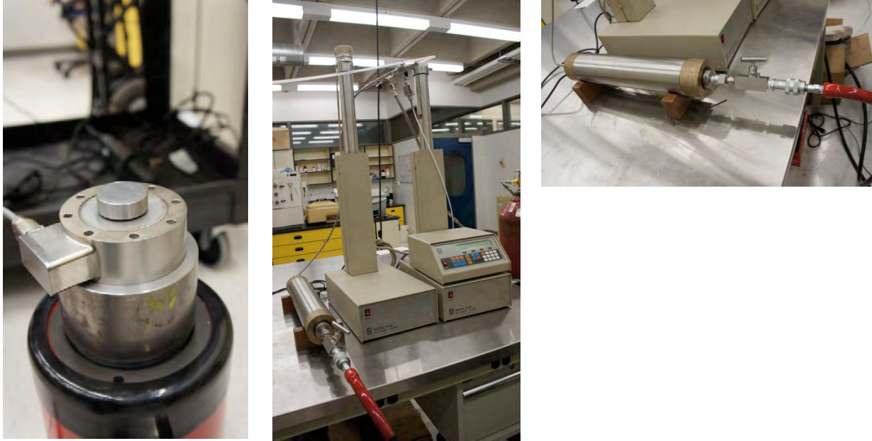
Figure 16: (left) Load cell mounted on top of the hydraulic jack. (middle) Isco pumps for precise pressurization of the jack and controlled application of axial load. (right) Accumulator that separates hydraulic fluid in the pump from the hydraulic fluid in the flexible hose for the jack.
