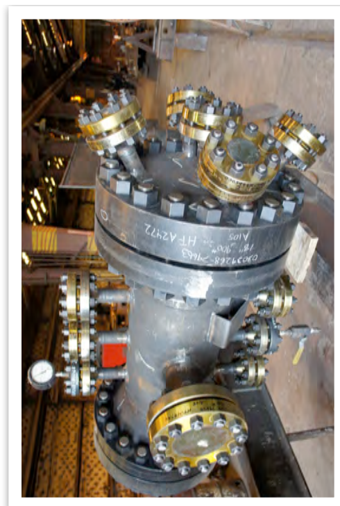
Figure 18: Schematic cross-sectional view and photograph of pressure vessel to be used for applying confining pressure.
