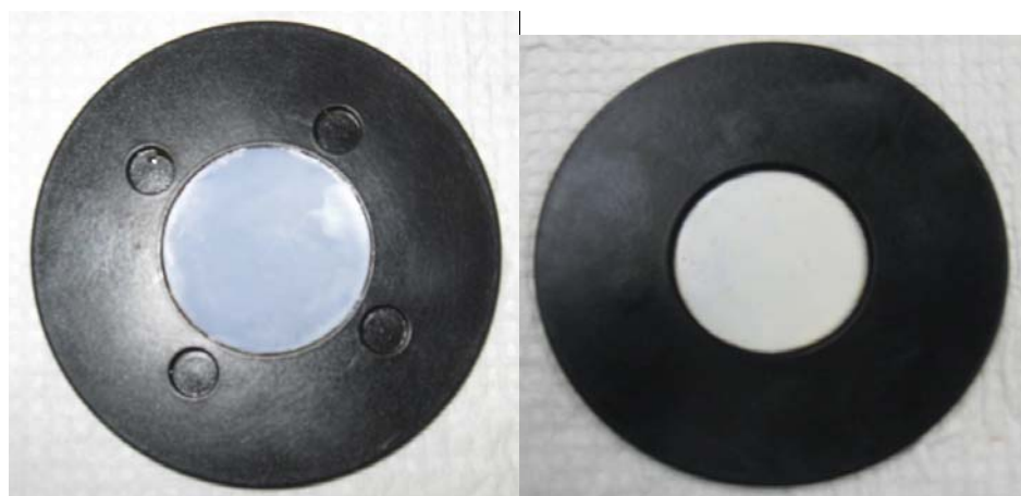
Figure 13. Anode [A] and Cathode [B] sides of the LiSICON 10B membrane after disassembly from Li Recovery Dual Flow Cell 20101029
