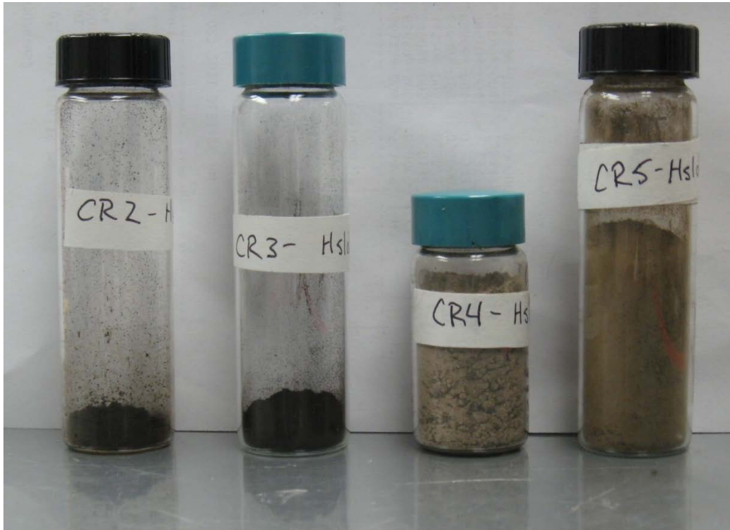
Figure 3: Picture of the dried solid samples of two nitrogen Coker Diesel runs (CR2, CR3) and two Coker Diesel hydrogen runs (CR4, CR5)
