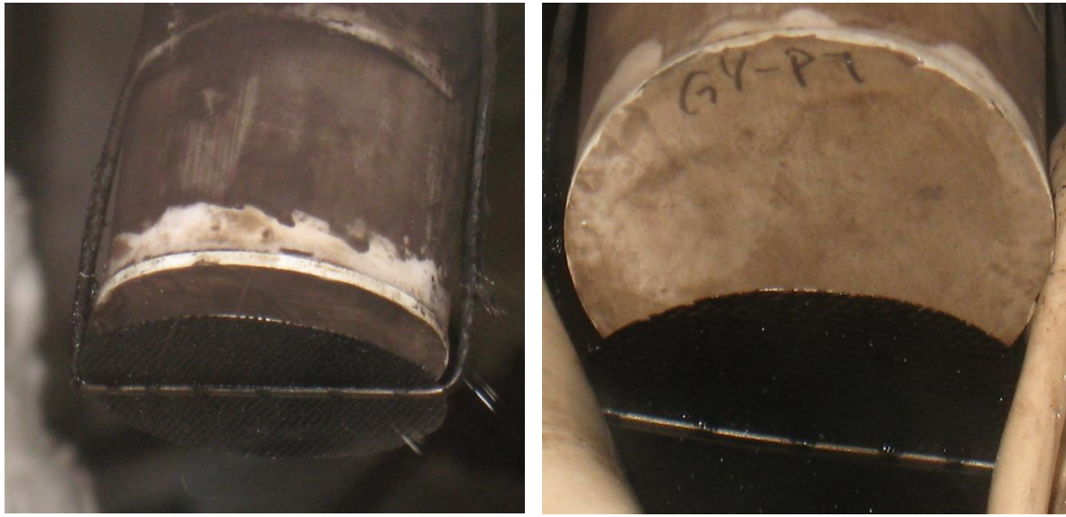
Figure 11. Platinized Ti electrode [A] and anode side surface of NaSICON-GY membrane [B] of Test Cell Molten Na_Bitumen_DL07_180-189-183+JK03004_20110808 after the test
