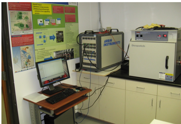
Figure 7. 16-channel Potentiostat/Galvanostat Arbin BT2000 instrument and lab oven installed in the Electrolytic Lab
