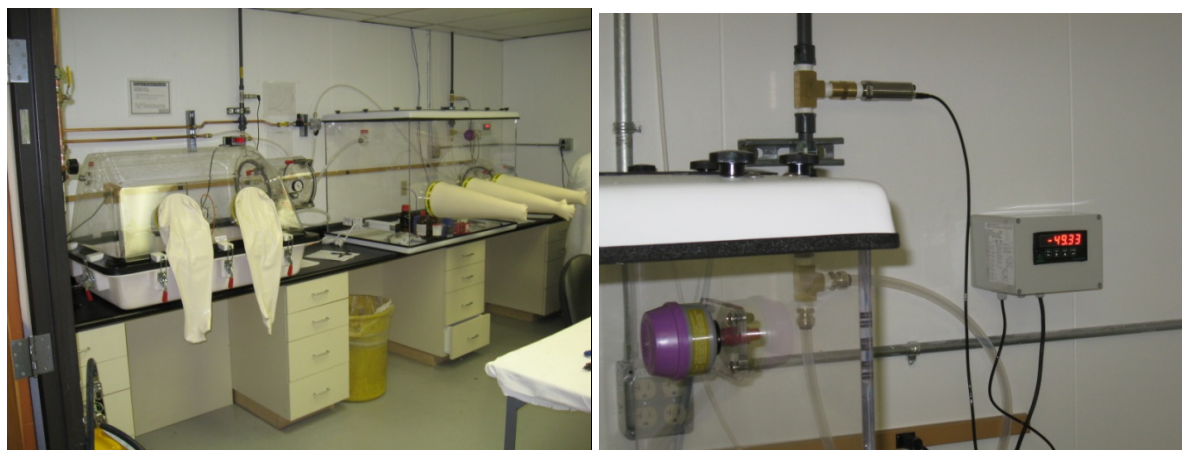
Figure 6. [A] Dry glove boxes in the Electrolysis Lab [B] New moisture sensor installed on the exhaust pipe of the new glove box
