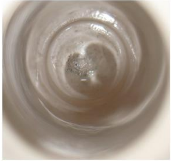
Figure 10: Anode [A] and cathode [B] sides of cell Na_molten_20110202 at the end of the run after 270 hours of operation
