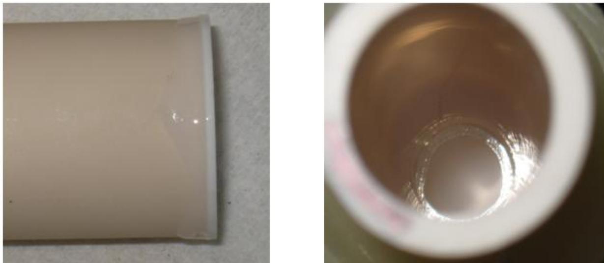
Figure 5: Anode side [A] and cathode side [B] of a Molten Sodium Recovery Cell showing the glass seal
