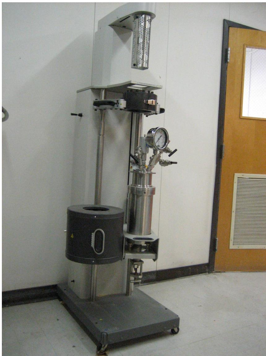
**Figure 2: New reactor for continuous operation**
