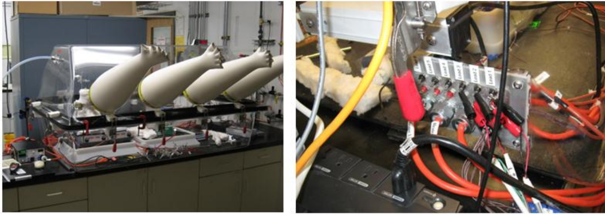
Figure 4: . Front of view of new 41ft 3 Plas-Lab acrylic glove box [A]. Side panel with feed through connections for heaters AC power, cells DC power, and type T thermocouples [B].
