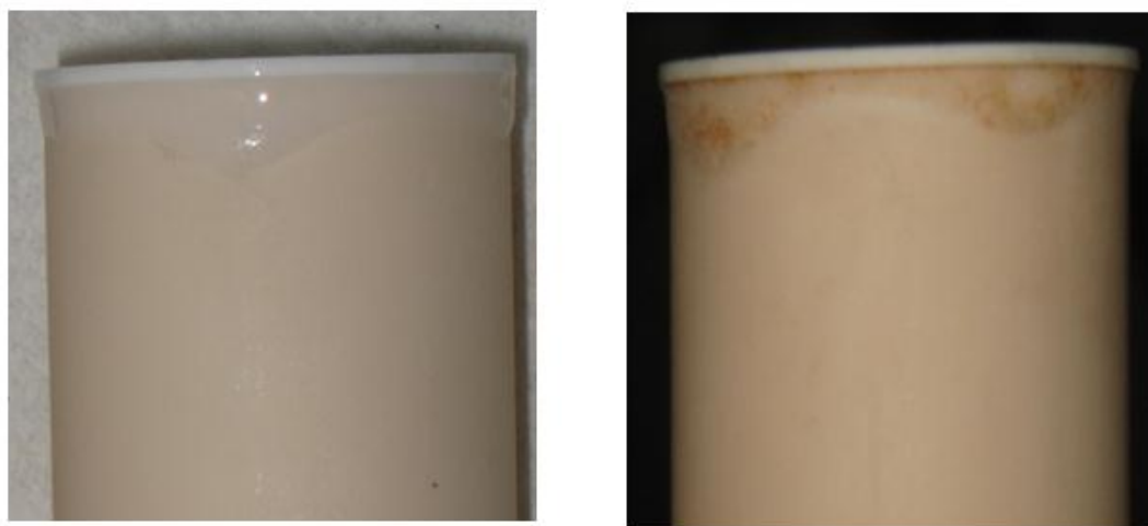
Figure 13: Glass seal before [A] and after [B] run of cell NaOH_EG_Molten_Na_20110411
