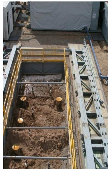
Figure 4. Cellar showing various conductor pipes for wells. Also shown is the rail system for moving the rig.
