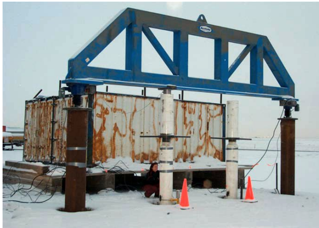
Early tests of design of spiral legs for platform foundations (UAA, “Tundra Platform Leg Tests,” Feb. 2003)
