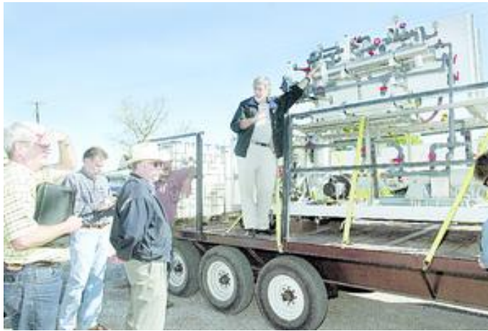
Texas A&M University's Global Petroleum Research Institute prototype oilfield-brine desalination unit in McFaddin Texas. The unit will be tested in August at McFaddin's Rio Vista Bluff Ranch, which will use the fresh water produced
