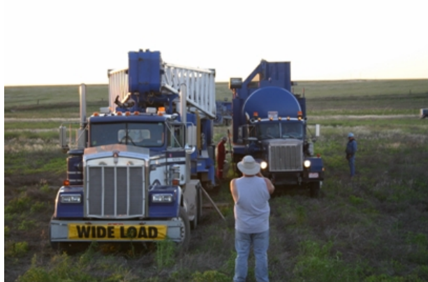
Figure 11 - Operator Trailer aligned next to the Rig Trailer.
