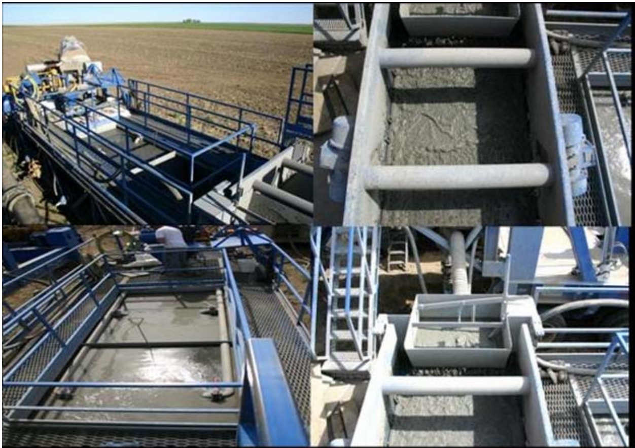
Figure 17 - Mud Tank Trailer, Mud Shaker and Zero Discharge Mud System
