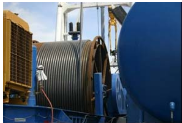
Figure 7- Coiled Tubing Drilling Rig Reel Mounted on the Rig Trailer
