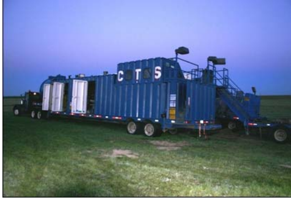
Figure 10 - The Operator Trailer controls and provides power to the Drilling Rig
