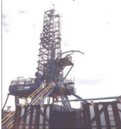
Figure 29: CTD Unit Mast and Substructure for CT Sizes through 5½ in.
