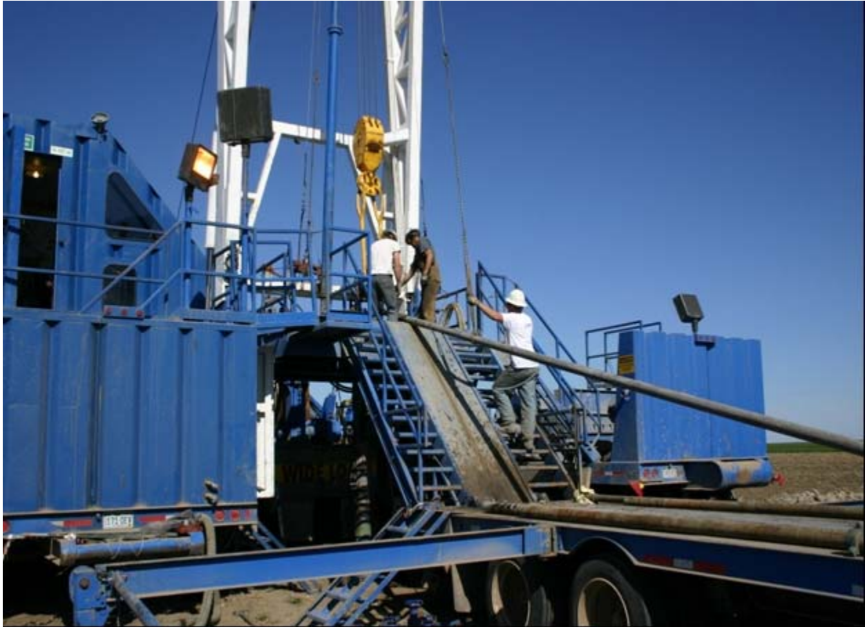
Figure 21 - Coiled Tubing Drilling Rig handling Casing without Extra Equipment
