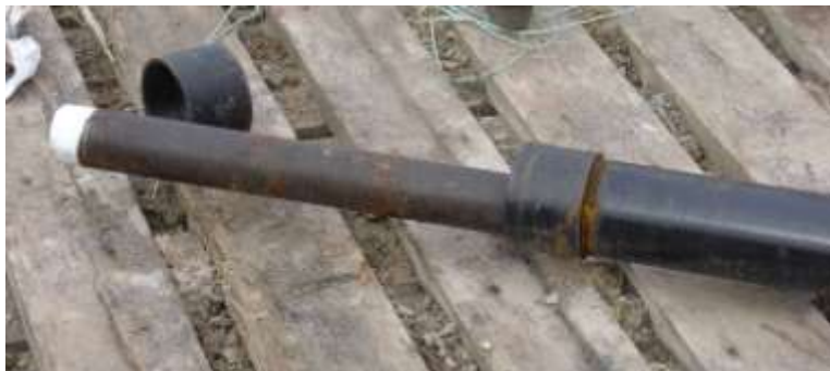
Figure C-5. Pipe in pipe for mud line
