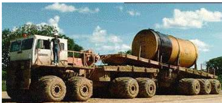
Figure 61: Rolligon Vehicle with Low Ground Pressure (4.4 psi) Transporting a Load of 100,000 lb
