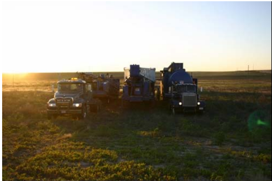
Figure 16 - Mud Trailer and Zero Discharge System Aligned Next to the Drilling Rig Trailer, on the left hand side of the photograph
