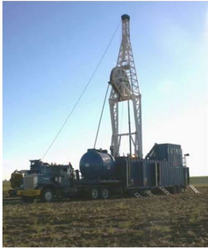
Figure 7- Coiled Tubing Drilling Rig Reel Mounted on the Rig Trailer
