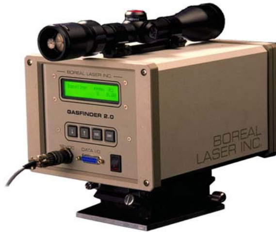
Figure 3. Boreal Laser TDL Transceiver
