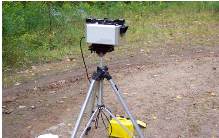
Figure 4. Example of TDL Transceiver in Field Position
