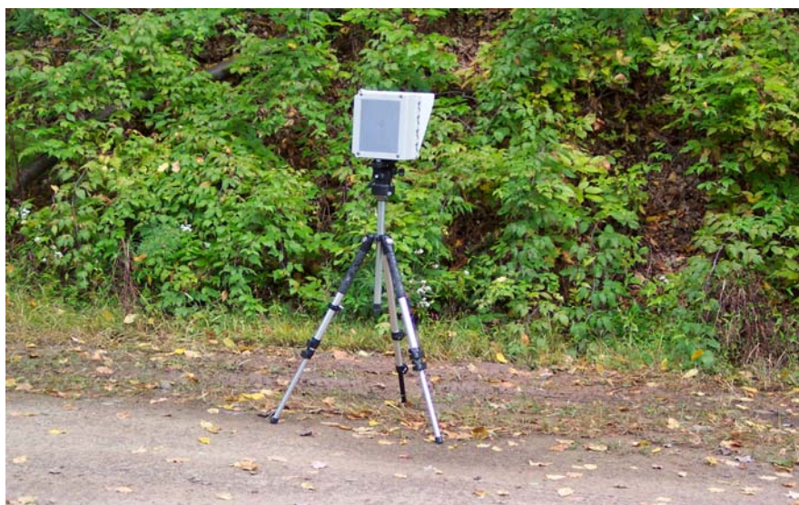
Figure 5. Example of TDL Retro-reflector in Field Position
