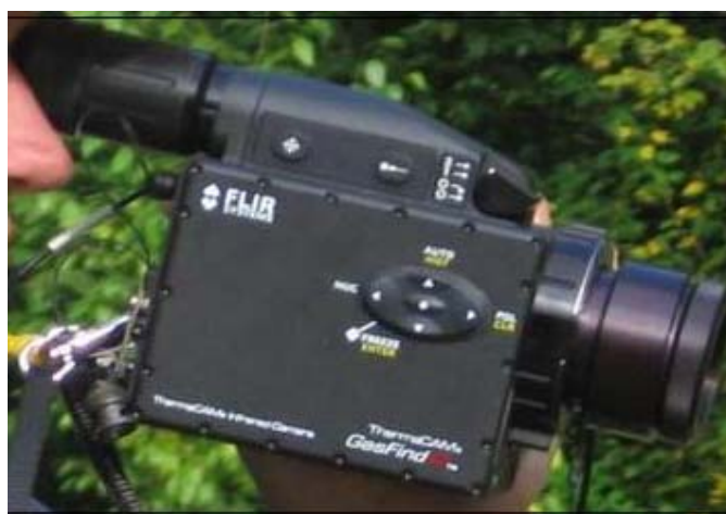
Figure 6. Infrared Video Camera Used for Spotting Emission Plume at Source
