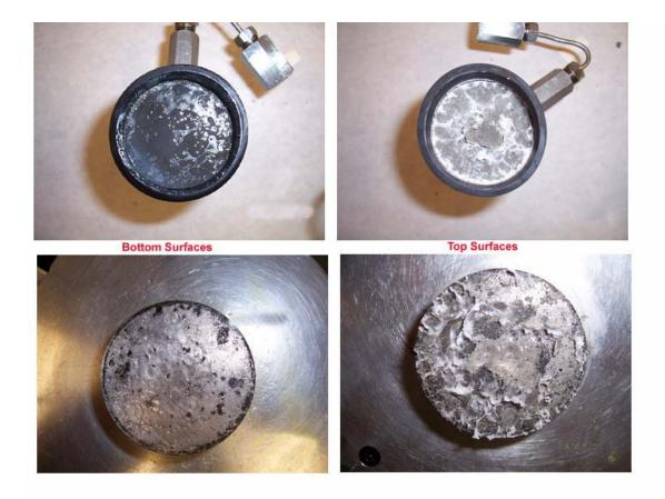
*Figure 7.* Post test photographs of top (right side) and bottom (left side) surfaces of test specimen (top) and end platens (bottom).
