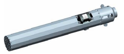
**Figure 34** 3D model of the circumferential subassembly. Suspension capability in the nose cone can be seen in the upper right.
