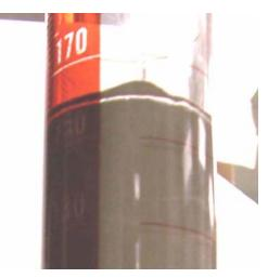
Figure 4. Side view of a graduated cylinder (250 ml) filled with cement slurry, after curing overnight. The white line around the circumference at the top of the cement column delineates the zone initially occupied by water expelled from the cement, and later re-absorbed
