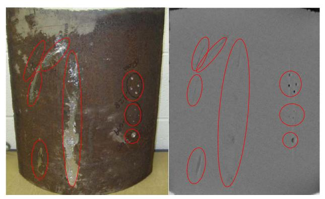
Figure 26. Sample scan of ¼ inch wall steel pipe, 160 kV; similar to Figure 7-4 with additional optimization.
