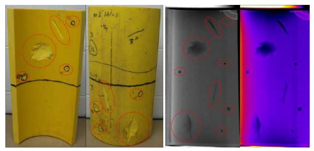
Figure 29. Sample RSD scan of MDPE, 12 inch diameter, DriscoPlex 6500 PE 2406 (1 mm pixels and 2.469 ms/pixel).
