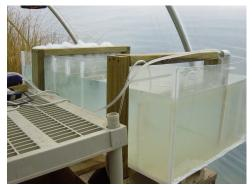
Figure 27: Newly constructed Oil/Water Separator used in Experiment 4.
