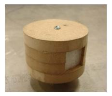
**Figure 21** 4-layer MDF block inserted into the prototype skeleton to provide a mild force to keep the EMAT sensors against the pipe wall.
