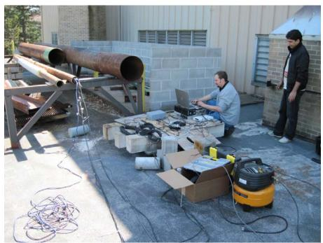
Figure 38 Experimental setup at Penn State for tests on 4" schedule 40 well casing.
