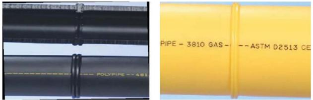
Figure 33. Acceptable butt fusion welds – proper alignment and double roll-back bead
