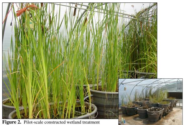
System (CWTS) for water produced from natural gas storage. The smaller photograph shows the system in its early stage of construction. The two trains on the left are the freshwater wetland cells that form the final stage of treatment. The two trains of wetland cells on the right contain *Spartina alterniflora*, which is used for the treatment of saline water. The larger photograph shows the CWTS in June 2005 following the successful establishment and growth of the wetland plants.
