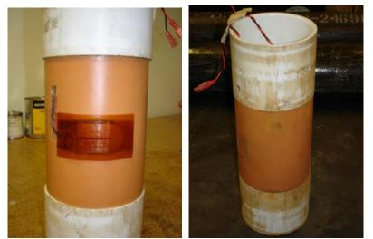
**Figure 22** Left: 1<sup>st</sup> generation tool with sensors installed. Right: after installation of the wear-resistant coating.
