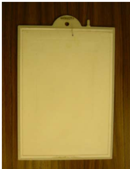
Figure 3-7. Ultrasonically welded polyethylene membrane sheet on an ABS plastic housing. Membrane was provided by Enviroquip, Inc. (Austin, TX).
