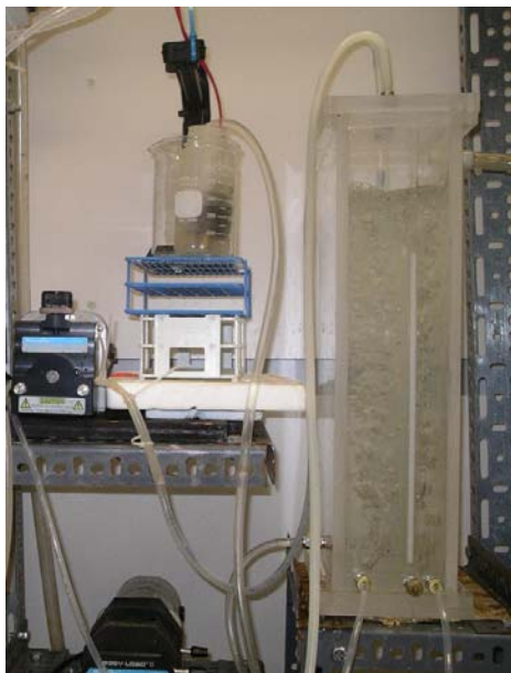
Figure 3-6. Experimental MBR system
