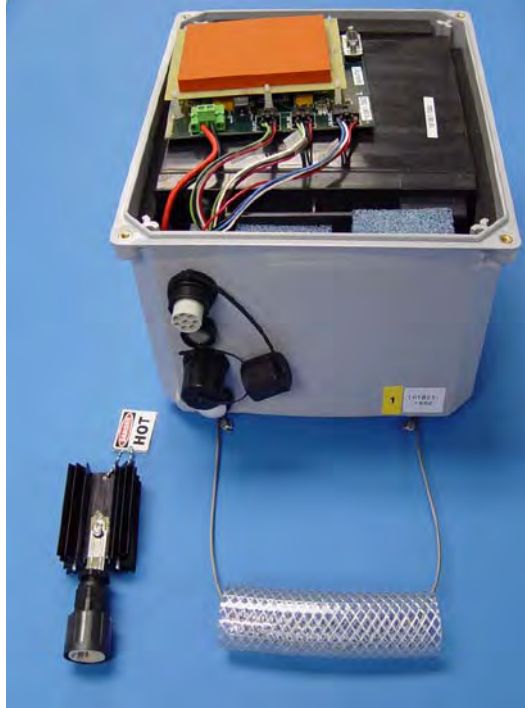
Figure II-16: Battery power enclosure with discharger
