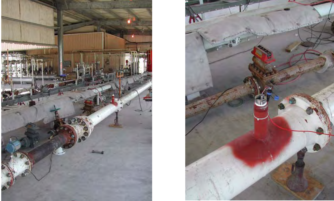
Figure II-24: SwRI Metering Test-Loop Calibration Setup
