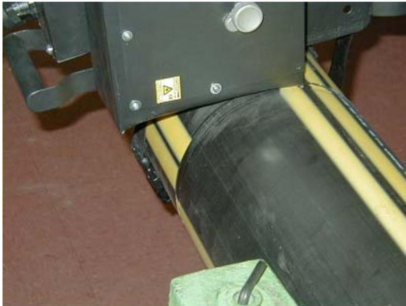
**Figure 24. WZIM Inspection Tool Performing Laser Scanning Process**
