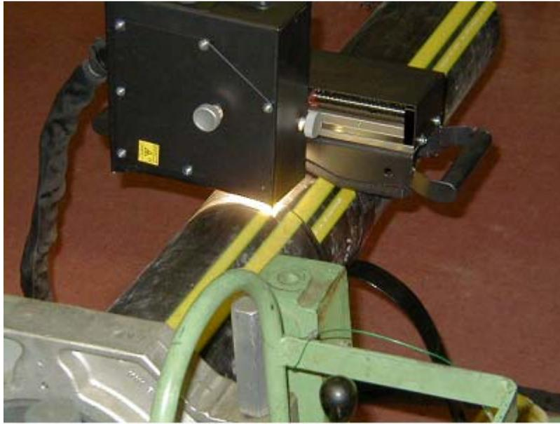
**Figure 23. WZIM Inspection Tool Performing Local Reheating**
