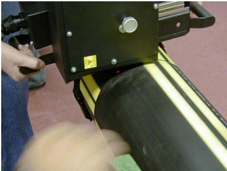
**Figure 22. Placing WZIM Inspection Tool on Pipe**
