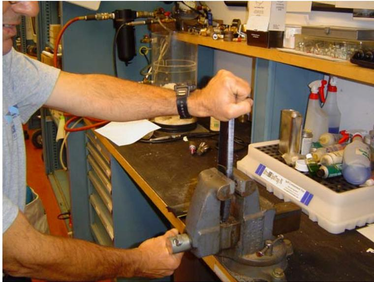
**Figure 35. Operator Performing a Destructive Bend Test on a Piece of Weld Joint Cut from a Pipe Inspected using the WZIM Tool**
