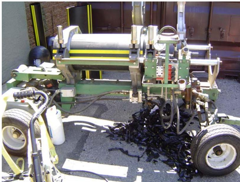
**Figure 32. HDPE Pipe in Fusing Machine at ConEdison Facility**
