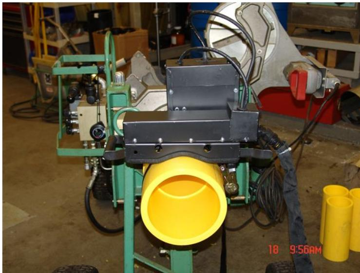
Figure 65. WZIM Inspection Tool on 8-in. MDPE Pipe during Field Trials with KeySpan
