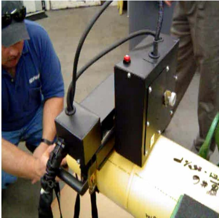
**Figure 62. Operator Awaiting Results from WZIM Inspection using Tool on MDPE Pipe at KeySpan Facility during Field Trials**
