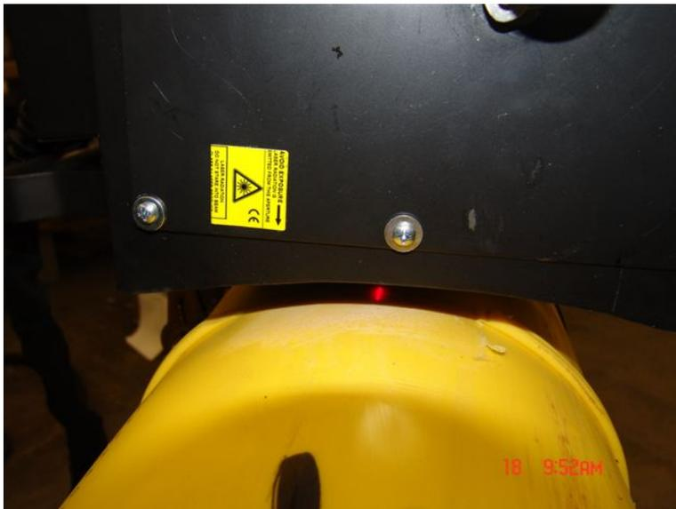
**Figure 63. WZIM Inspection Tool Performing Laser Scanning Sequence during Field Trials at KeySpan Facility**
