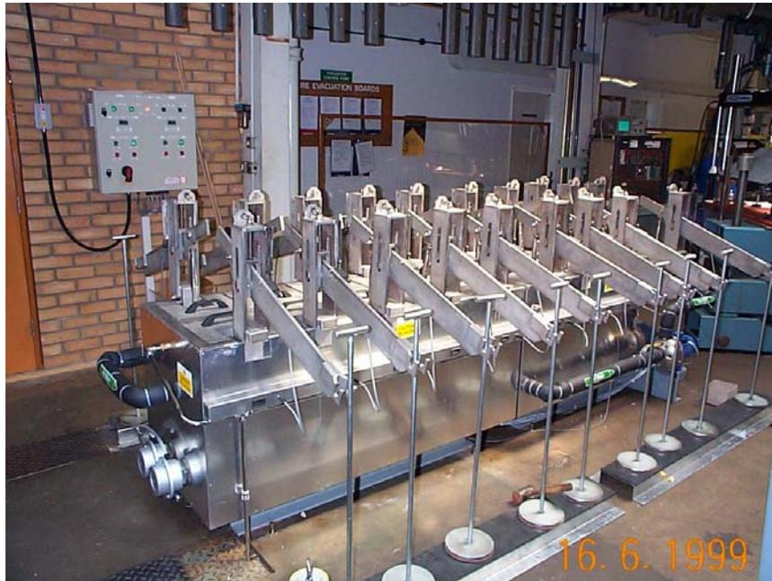
**Figure 15. Photograph of Tensile Creep Rupture Test Rig**
