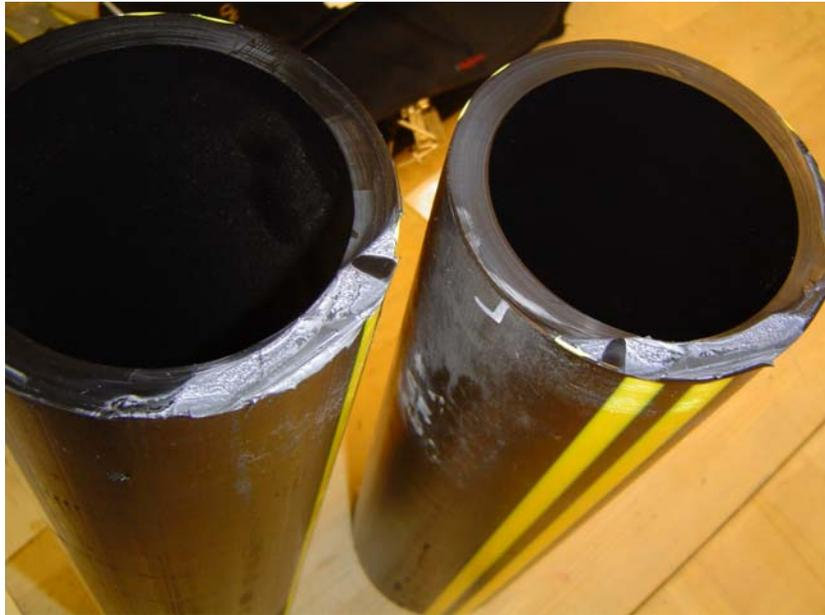
**Figure 84. Cold Weld Defect on Small Section of Joint Interface** (Notice that the cold weld defect does not exist over the entire joint.)
