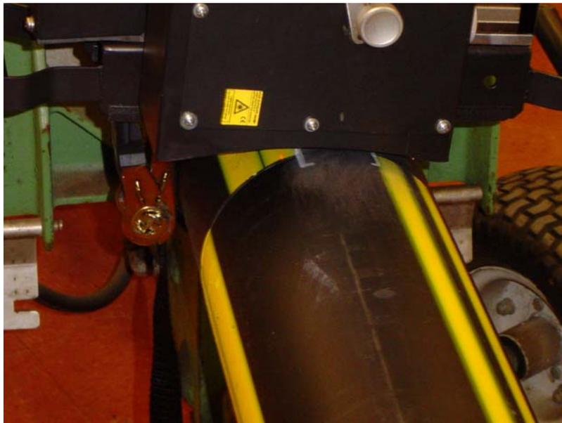
**Figure 34. WZIM Inspection Tool Performing Inspection at ConEdison Facility during Field Trials**
