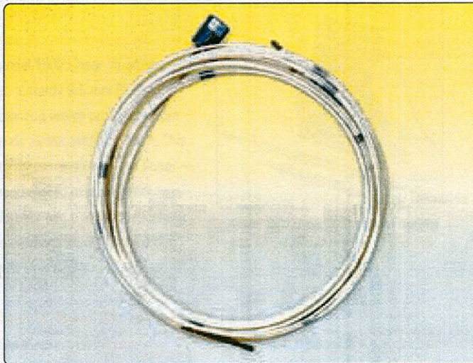
• Model A-6 assembled with groutable anchors and coiled for shipment.
