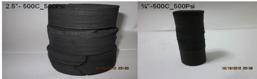
**Figure 22:** Images of the spent shales from two different scales pyrolysis. Sample on left is 2.5” core, sample on right is 3/4” core.
