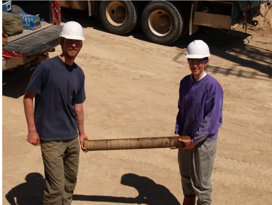
Figure 7: Section of 4-inch core.
