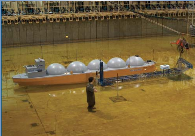
Figure 2. Bluewater Offshore's "Big Sweep" undergoing wave tank model testing.
