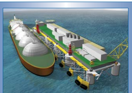
Figure 6. FMC Sofec Offshore's liquefied natural gas mooring system.
