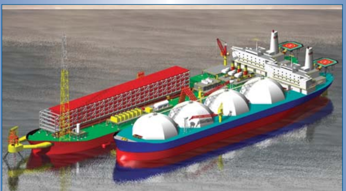
Figure 5. SBM-Imodco Offshore's liquefied natural gas mooring system.
