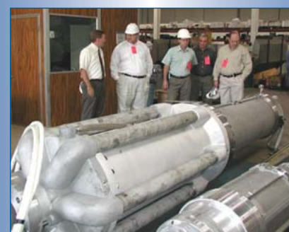
Figure 8. Ebara's liquefied natural gas pump in assembly.
