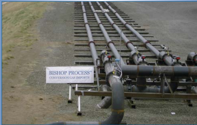
Figure 10. The Bishop Process heat exchanger being field tested.
