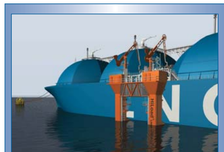
Figure 7. Remora Technology's "Hi Load" liquefied natural gas mooring system.
