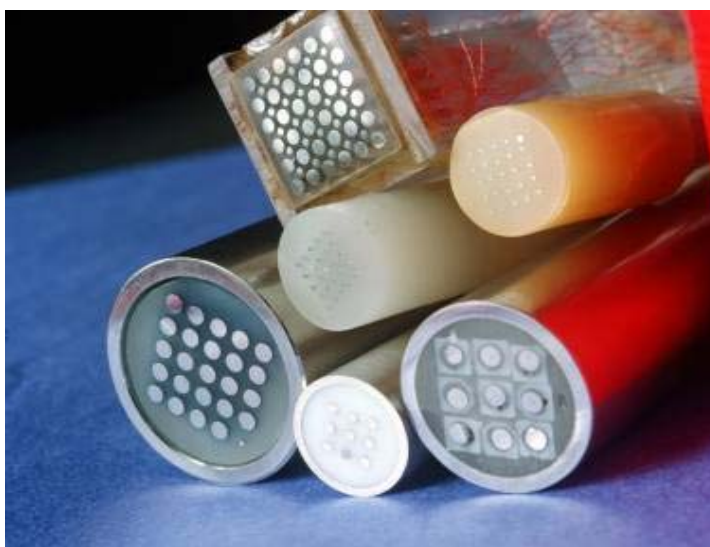
Figure 5: End view of several different versions of the SwRI developed MAS probe.
