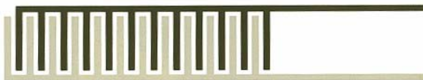
Figure 4: Planar view of thin film interdigitated galvanic couple sensor. This sensor is currently composed of conductive carbon (black lines) and silver laid out on Mylar.
