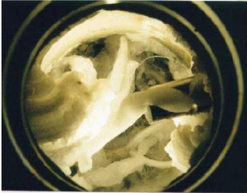
Fig. 9. Developed growth of hydrate crystals--pure water/ethane
