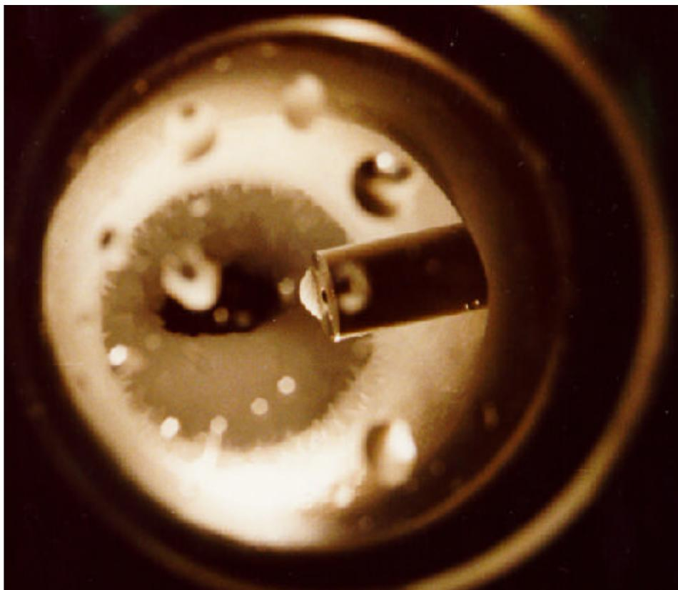
Fig. 11. Developed growth of hydrate crystals--surfactant/water/ethane, Run #34.
