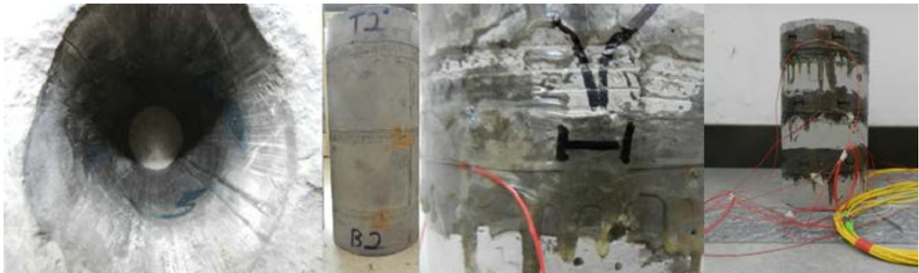
Figure 2.8.4. Experimental design for fiber optic monitoring of a SCARC specimen.
