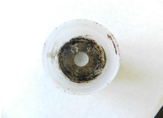
Figure 2.8.13. Specimen with cored reservoir.
