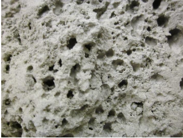
Figure 2.8.4. Porous concrete sample formed in Shen-En Chen's laboratory at UNCC, for simulation of rock formations saturated with oil, water, and CO 2 having different strengths and stiffness.
