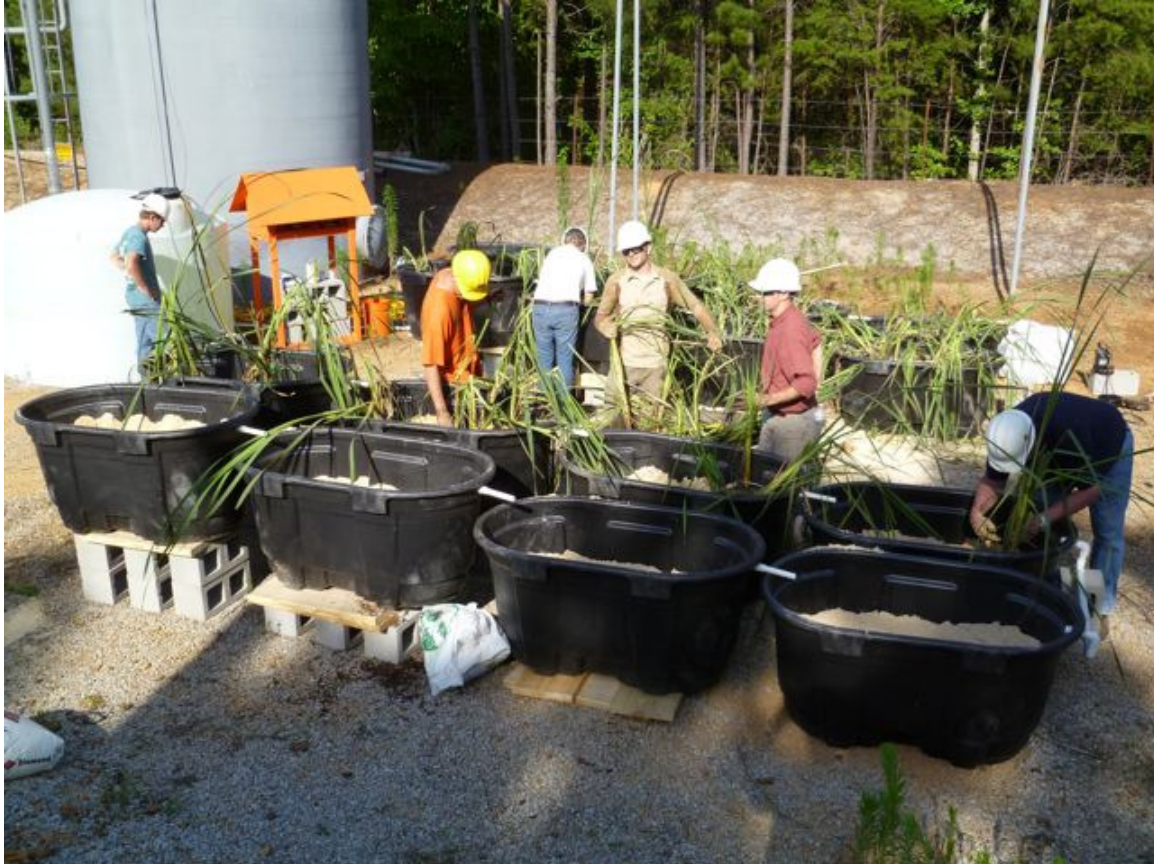
Figure 60. Broadleaf and narrowleaf cattails ( Typha latifolia and Typha angustifolia ) were collected from a nearby pond and transplanted to the demonstration CWTS cells at a density of 30 plants per cell.
