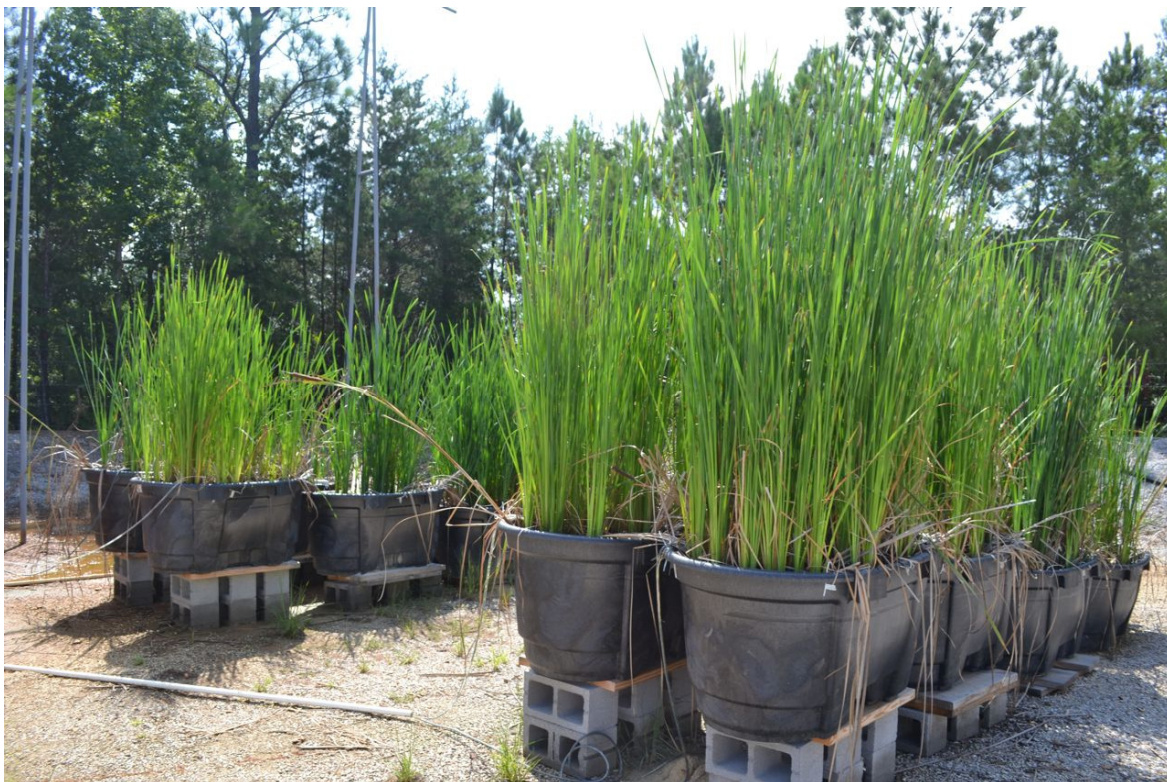
Figure 69. Demonstration wetland treatment system on 9/7/12, 14 weeks after construction.
