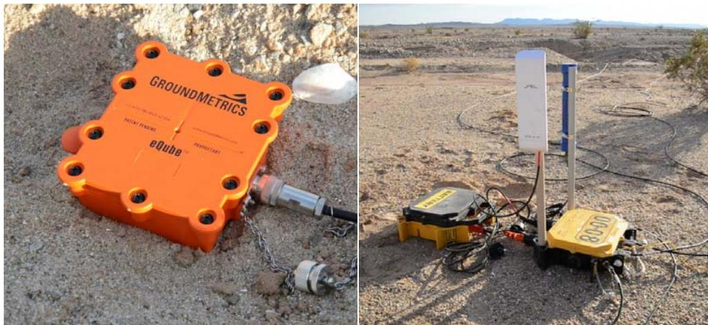
**Figure 4. GMI sensing equipment. Left: Most recent GMI eQube sensor. Right: GMI data acquisition units.**
