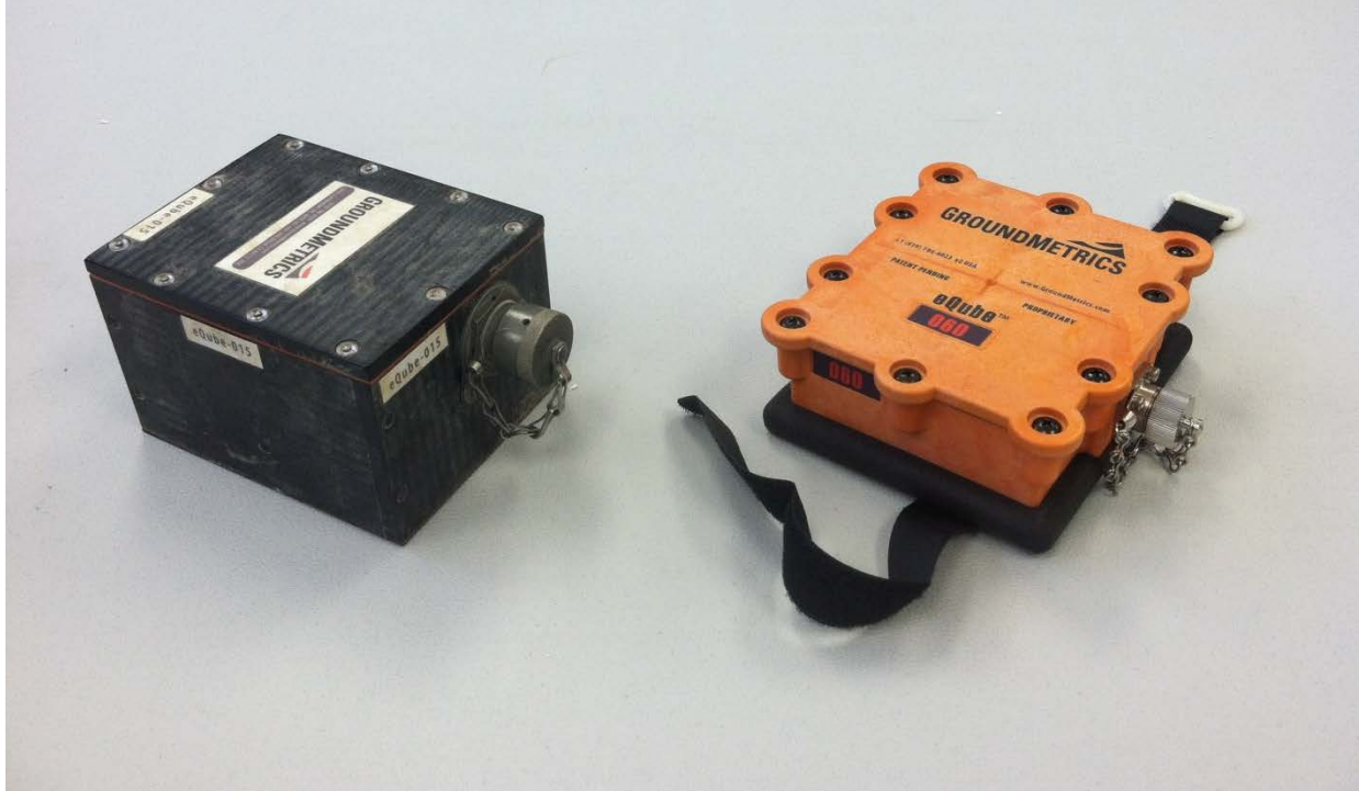
Figure 14. Old (left) and new (right) version of GroundMetrics e-field sensors
