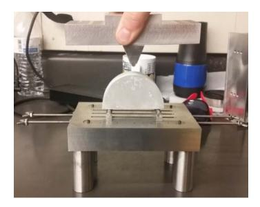
**Figure 2.** Photograph of three-point bending fixture. A customized loading fixture is used in a servo-controlled loading frame to apply axial load. This particular sample does not have a starter crack.
