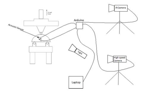
**Figure 1.** Task 6 experimental setup. The three-point bending fixture has been adapted to fit into a servo-controlled load frame. The starter notch is shown. As the load is applied to the notched sample, acoustic activity is measured. With an acceleration in acoustic emissions, the high-speed camera is tripped and the high-speed and IR cameras are fired and information is stored on the laptop.
