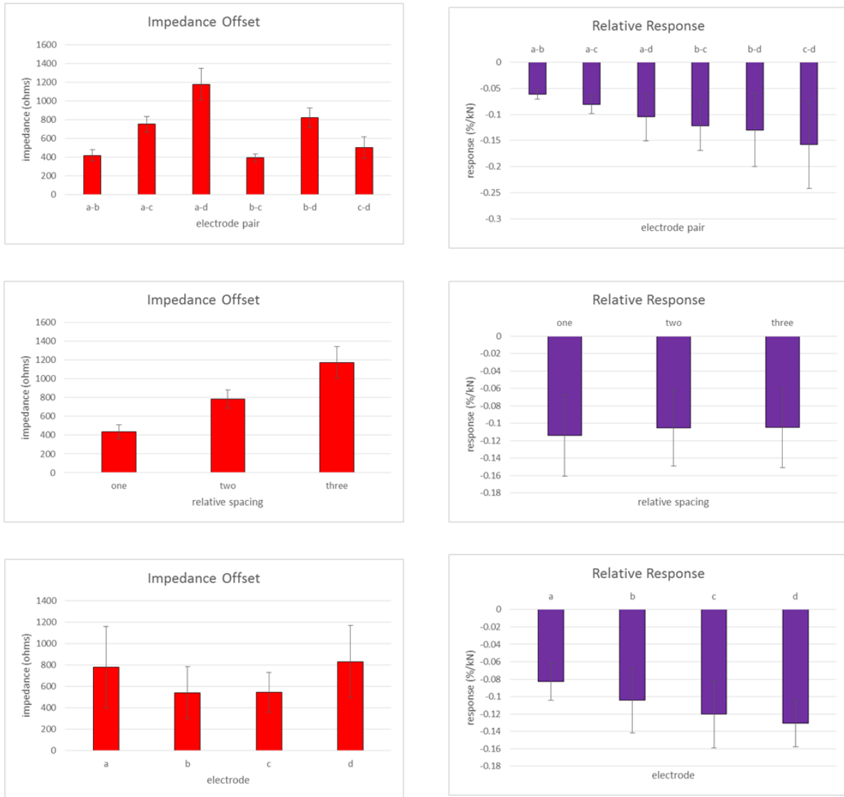
Figure 81: Impedance offset (left) and relative impedance response to load (right) for electrode pairs (top), electrode spacing (center), and individual electrodes (bottom).
