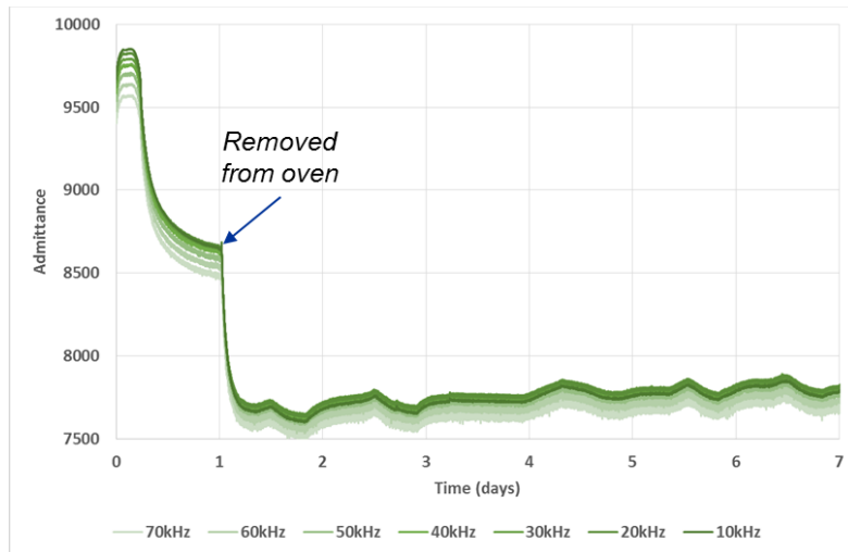
Figure 27: Nanite raw electrical impedance data collected for a range of frequencies over the first week of curing.
