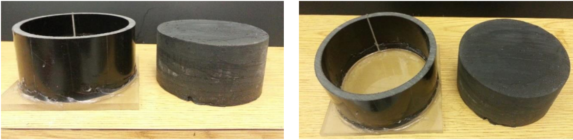
Figure 25: Samples for chloride ion permeability testing.
