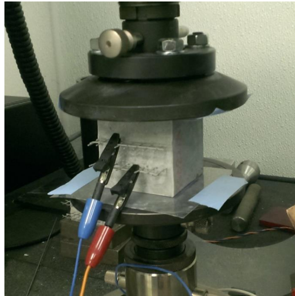
Figure 69: Nanite 2" cube specimen with grid electrodes under test
