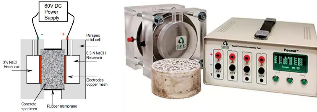
Figure 24: Rapid chloride permeability cell (left) and system (right).
