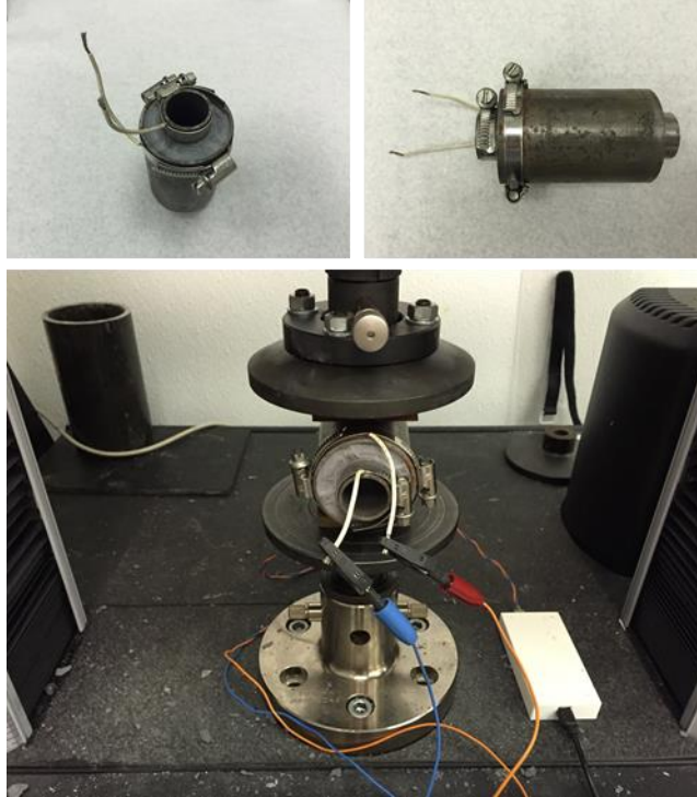
Figure 48: Concentric pipe with cement sheath form factor for testing Nanite (top). Cemented concentric pipes connected to the impedance analyzer in the Instron for resistivity-load measurements
