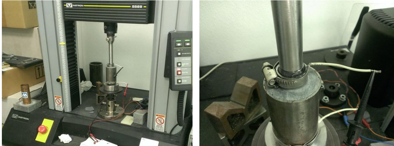
Figure 58: Pipe expander testing with Instron machine
