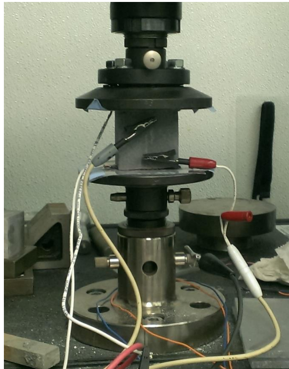
Figure 75: 4-wire Electrical Impedance Testing using copper surface electrodes and gel couplant.
