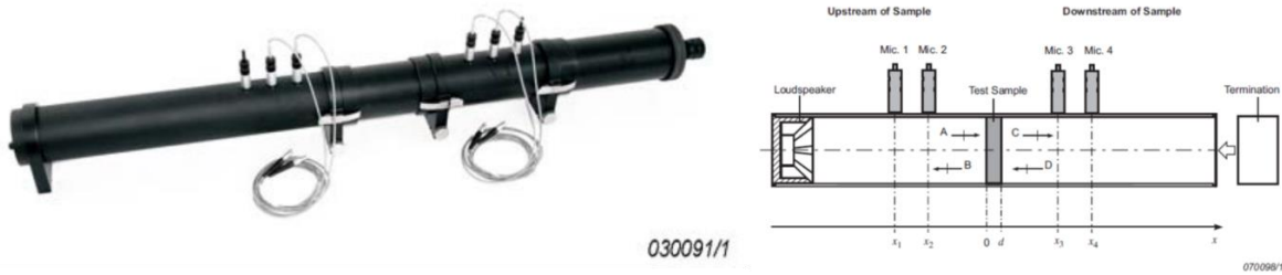
Figure 36: Acoustic impedance tube (left) and schematic of sample and microphone setup (right).
