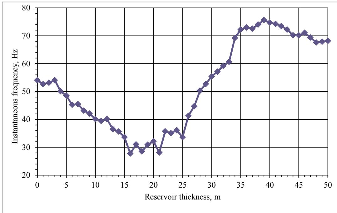
Figure 4.22. Crossplot of the RMS average instantaneous frequency within a 5ms window centered at Reflection\_1 (interpreted on the synthetic seismic section built at well #15-191-22591, Figure 4.18) versus the reservoir thickness.
