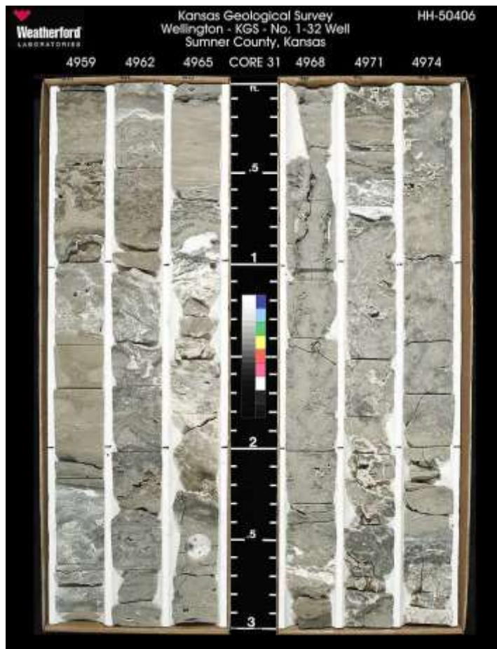
Figure 27 Example of the carbonate facies and porosity in the injection zone in the lower Arbuckle(part of the Gasconade Dolomite Formation). Upper half is light olive gray, medium-grained dolomitic packstone with crackle breccia. Scattered subvertical fractures and limited cross stratification. Lower half of interval shown has occasional large vugs that crosscut the core consisting of a light olive gray dolopackstone that is medium grained. Variable sized vugs range from cm-size irregular to subhorizontal.
