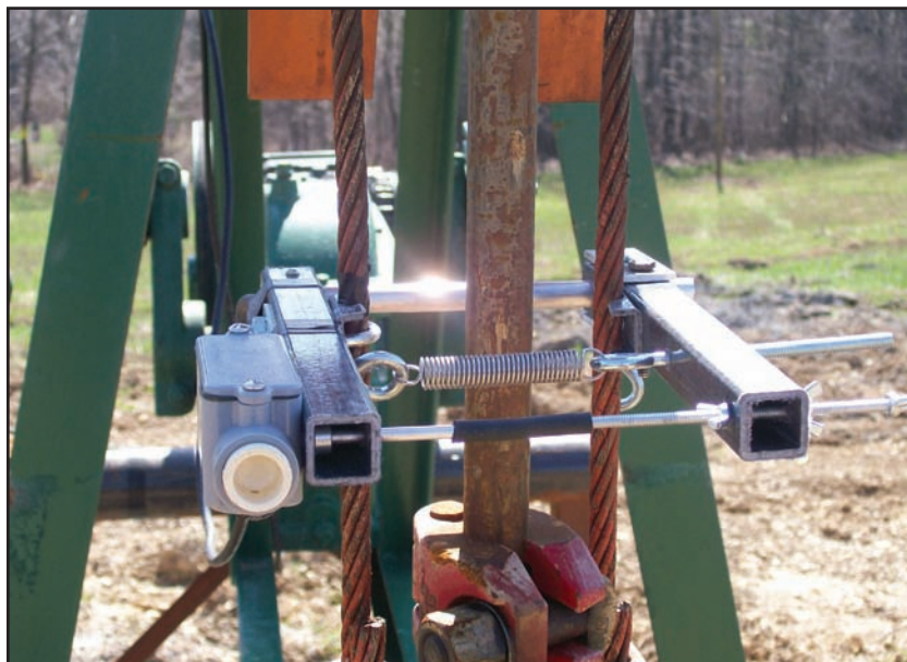
Figure 1. A fluid level sensor is mounted on the bridle cables below the horse's head.
