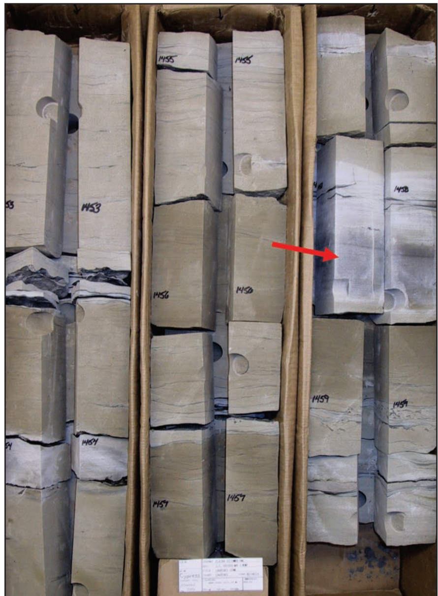
Figure 3. Core photograph, showing heterogeneity of the Lawrence Field reservoir rocks. Calcite cemented interval at red arrow has very limited porosity and permeability and forms a barrier to fluid flow.
