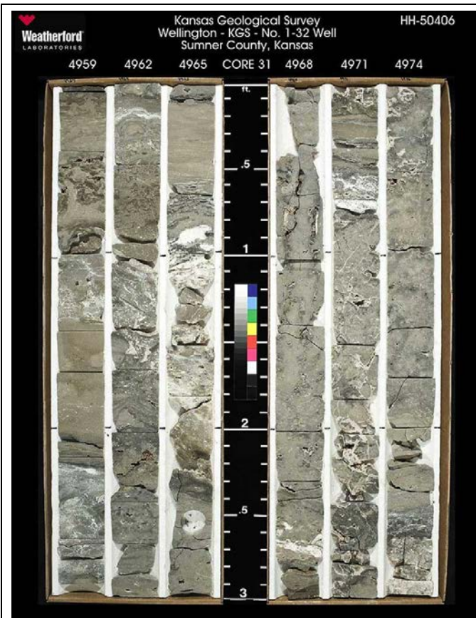
Figure 34. Example of the carbonate facies and porosity in the injection zone in the lower Arbuckle (part of the Gasconade Dolomite Formation). Upper half is light olive-gray, medium-grained dolomitic packstone with crackle breccia. Scattered subvertical fractures and limited cross stratification. Lower half of interval shown has occasional large vugs that crosscut the core consisting of a light olive-gray dolopackstone that is medium grained. Variable-sized vugs range from cm-size irregular to subhorizontal.
