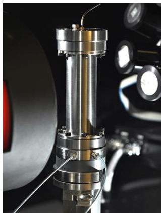
Figure 18: High-pressure beryllium chamber on the micro-CT station.
