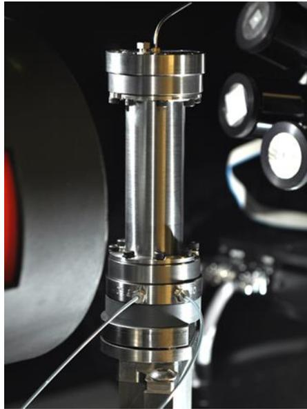
**Figure 33: High-Pressure Beryllium Chamber on the Micro-CT Station.**
