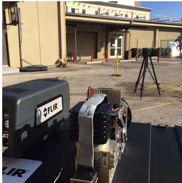
Figure 2: Niatros™ and FLIR MWIR Cameras Acquiring Data During a Supervised Methane Release
