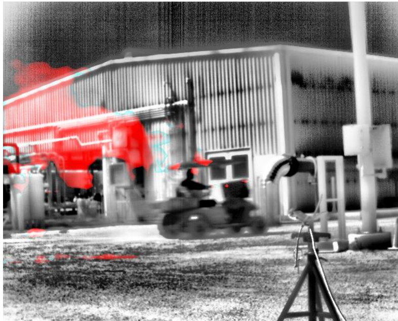
Figure 3: A dust cloud kicked up by a passing vehicle. The algorithm tries to classify some of the less opaque areas of the dust cloud that look like a plume.
