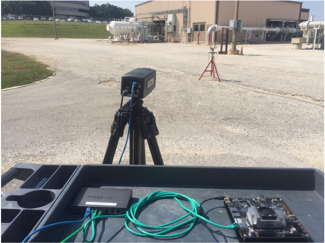
Figure 7: Test Setup for 9/13/17 Methane Release against SLED-M Software v1.4
